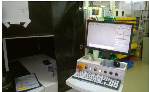
Fig. 5. Walter Helicheck Basic, optical CNC measuring machine
