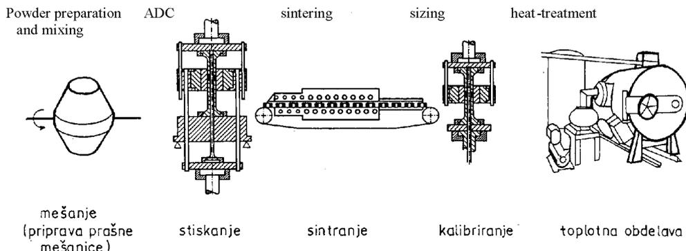
Figure 2: Schematic presentation of the phases of the conventional sintering process for the production of steel parts
