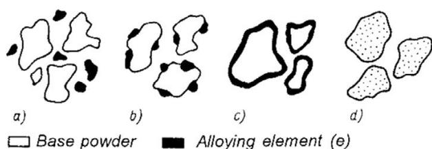
**Figure 9:** Standard ways of alloying techniques in powder metallurgy<sup>5</sup>
