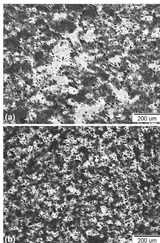
**Figure 12:** Microstructure of sintered and heat-treated gear: a) produced from original powder mixture and b) produced from fine sieved powder mixture; polished and nital-etched sample, light microscope, magnification 100-times
