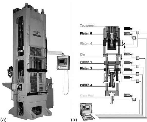
**Figure 5:** a) Modern hydraulic computer-controlled press for the automatic die compaction of steel powders and b) a schematic presentation of a multi-platen adapter system for the fixation of the tool into the press<sup>5</sup>
