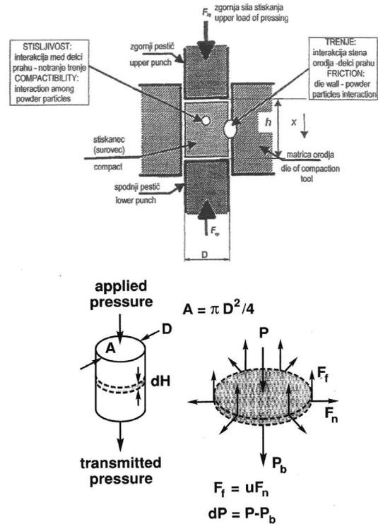
Figure 3: Schematic presentation and analysis of the uniaxial cold die compaction of metal powder in a cylindrical die<sup>6</sup>
