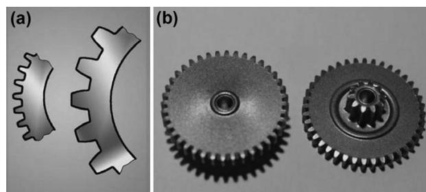
**Figure 6:** a) Schematic presentation of small and large gear module and b) a photograph of the discussed small complex double spur gear with the dimensions 5/40-7/10 x 7 mm, produced in the Sinter Workshop, Unior factory, Zreče, Slovenia
