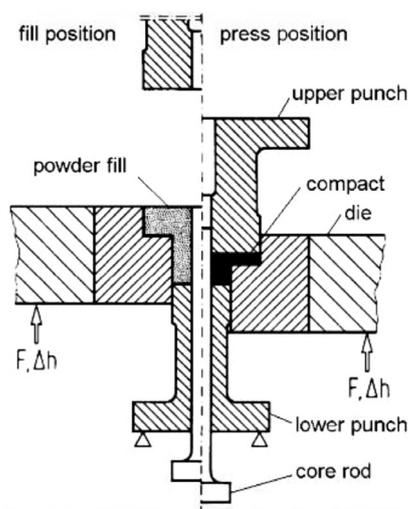
**Figure 7:** Schematic presentation of the cross-section of the tool for the uniaxial ADC of the double-height product<sup>5</sup>
