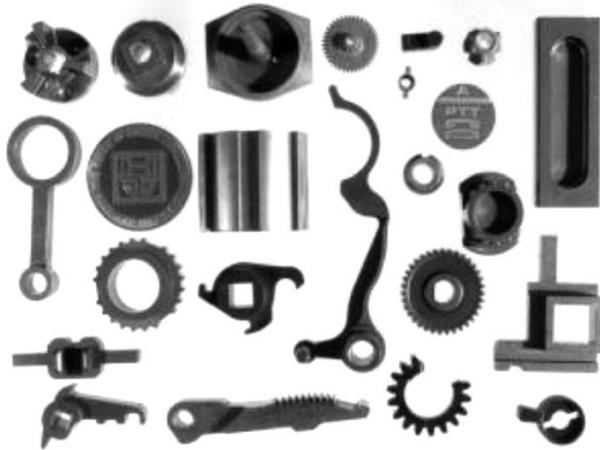
Figure 1: Some typical sintered steel parts
