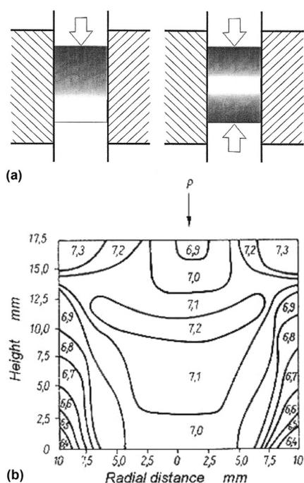
**Figure 4:** a) Schematic and b) practical presentation of the green-density distribution in a cylindrical specimen after the uniaxial cold compaction of steel powder<sup>5</sup>
