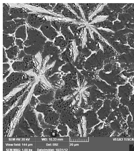
Figure 5: Microstructure of the water-quenched Al-7Fe-4Cu (SEM) Slika 5: Mikrostruktura Al-7Fe-4Cu po ohlajanju v vodi (SEM)
