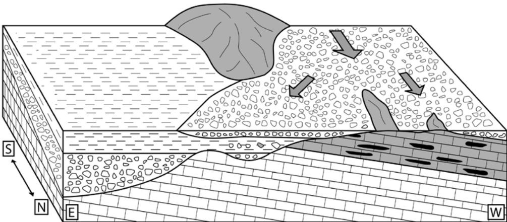
**Figure 5.** Schematic reconstruction of the »western basal limestone breccia« deposition (for details of reconstruction see the text for Figure 2)
