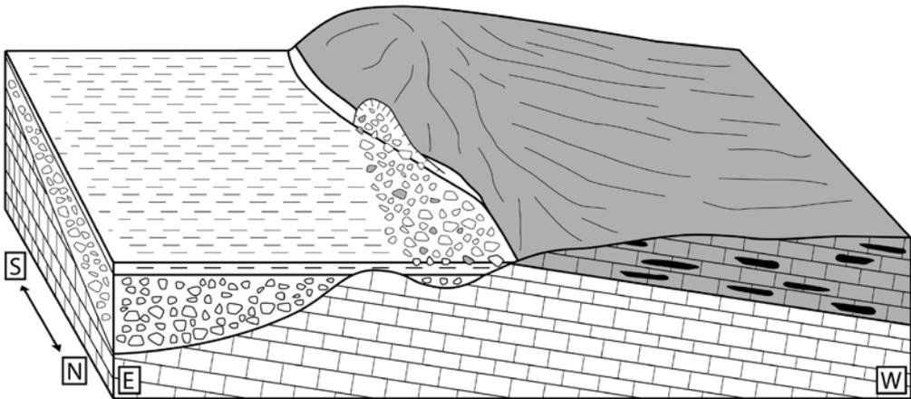
**Figure 4.** On-lapping of the flyshoid sediments (left) on the paleo-slope composed of Jurassic platform limestones (right)
