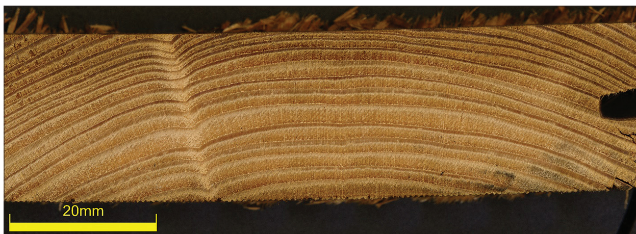
Figure 1. Cross-section of spruce wood plank, used for microscopic and sorption analysis.
