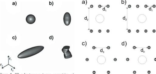
**Figure 1.** 3D subcutaneous tumor geometries. a) sphere  $(r_{1-3} = 2 \text{ mm})$ ; b) ellipsoid positioned deeper in tissue  $(r_1 = 4 \text{ mm}, r_{2,3} = 2 \text{ mm})$ ; c) ellipsoid  $(r_{1,2} = 2 \text{ mm}, r_3 = 8 \text{ mm})$ ; d) realistic tumor geometry from medical images  $(r_1 = 3.8 \text{ mm}, r_2 = 2.4 \text{ mm}, r_3 = 2.6 \text{ mm})$ .
