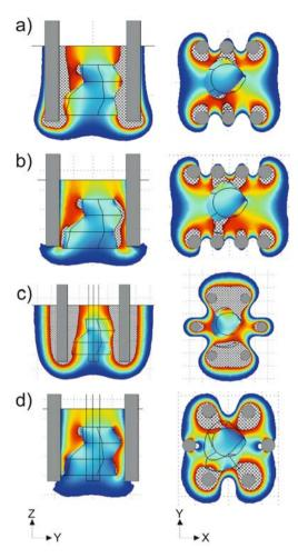
**Figure 5.** Electric field distribution for the optimized model of the realistic tumor with a) three needle pairs; b) four needle pairs; c) 3x3 hexagonal needle electrode array; d) 2x2x2 hexagonal needle electrode array is shown. The electric distribution is shown in two central perpendicular planes: YZ and XY both passing through the center of the tumor. Corresponding values of parameters are given in Table 1.
