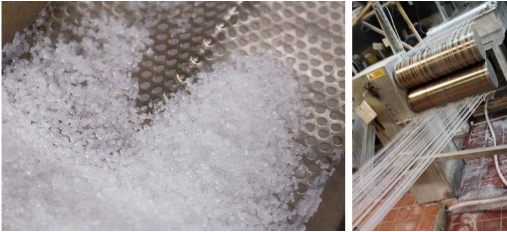
Figure 6: Manufacture of ECONYL® nylon granulates
