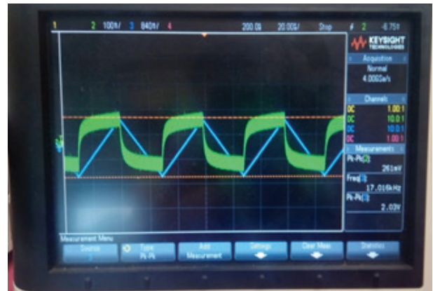
Figure 30: The experimental result of the inductor simulator
