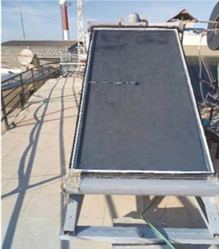
*Solar air flat plate solar collector*
