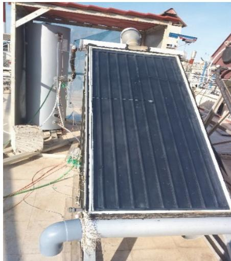
*Solar water flat plate collector with air absorber cooling*
