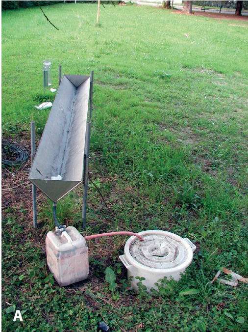
Slika 3a: Korita in b) totalizator za merjenje prepuščenih padavin Figure 3a: Throughfall and b) measurement with gutter and totalisator.
