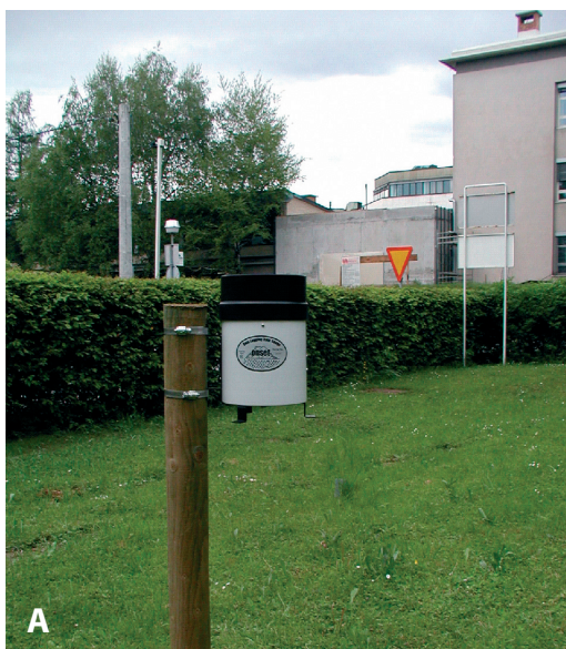
Slika 2a) Ombrograf Onset RG2-M in b) Helmanov dežemer za merjenje padavin na prostem Figure 2a: Onset RG2-M and b) Helman rain gauge for measuring gross precipitation.
