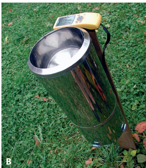
Slika 2a) Ombrograf Onset RG2-M in b) Helmanov dežemer za merjenje padavin na prostem Figure 2a: Onset RG2-M and b) Helman rain gauge for measuring gross precipitation.
