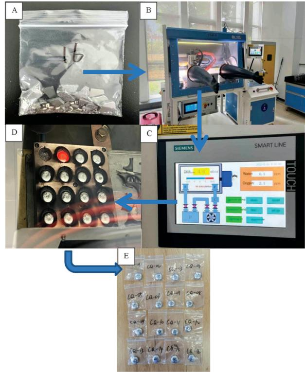
**Figure 1:** High-flux material multi-crucible synchronous smelting system: a) high-purity metal block raw materials; b) high-throughput preparation system; c) control interface; d) multi-crucible synchronous metallurgical platform; e) as cast metal ingots with different compositions
