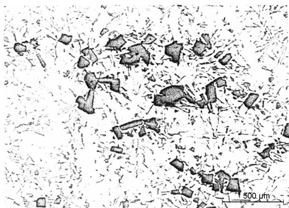
Figure 4: Microstructure of ring carrier (Inhomogeneous Si thinning) (100X)
