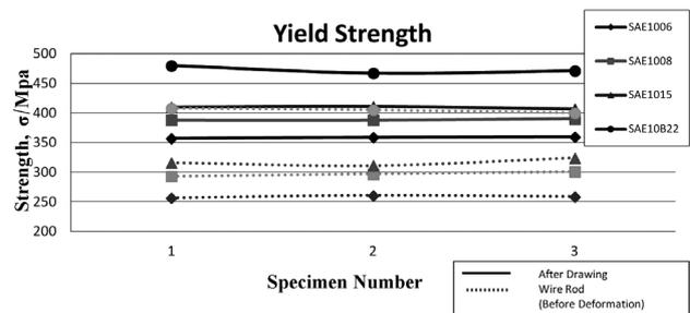
**Figure 4:** Variation in the yield-strength values for a rod and coil steel wire at a constant velocity and reduction ratio (from  $\phi 5.50$  to  $\phi 4.81$ )
