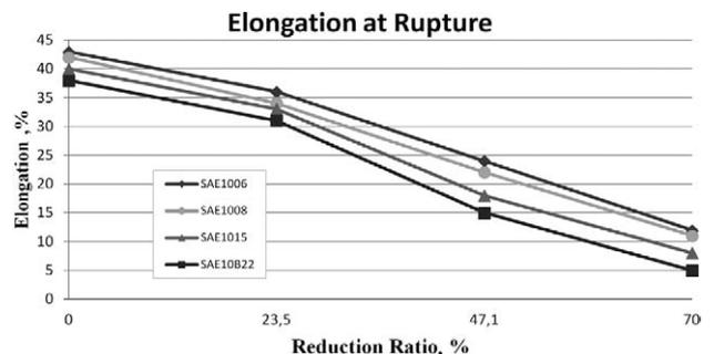
**Figure 11:** Variation in the elongation-at-rupture (%) values for a rod and coil steel wire at a constant velocity and different reduction ratios (from  $\phi 5.50$  to  $\phi 4.81$ ,  $\phi 4.00$  and to  $\phi 3.01$ )
