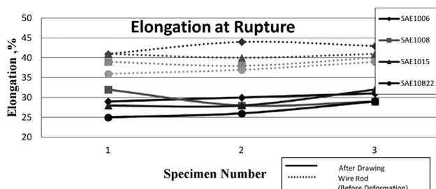
**Figure 6:** Variation in the elongation-at-rupture (%) values for a rod and coil steel wire at a constant velocity and reduction ratio (from  $\phi 5.50$  to  $\phi 4.81$ )
