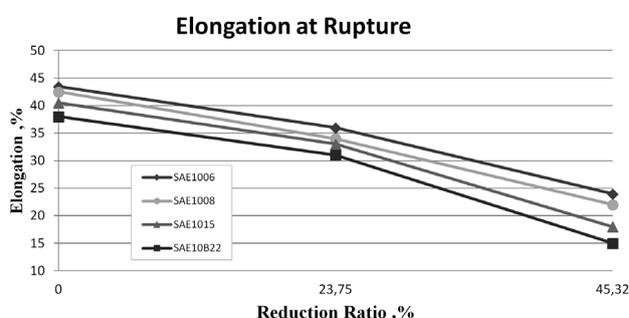
**Figure 14:** Variation in the elongation-at-rupture (%) values for a rod and coil steel wire at a constant velocity (3.6 m/s) and different reduction ratios – different inlet diameters and constant outlet diameters (from  $\phi 5.50$  to  $\phi 4.81$  and from  $\phi 6.50$  to  $\phi 4.81$ )
