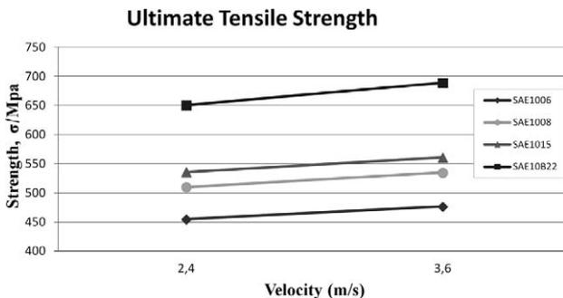
**Figure 16:** Variation in the ultimate-tensile-strength values for a coil steel wire at a constant reduction ratio (from  $\phi 5.50$  to  $\phi 4.81$ ) and with different drawing velocities (3.6 m/s and 2.4 m/s)
