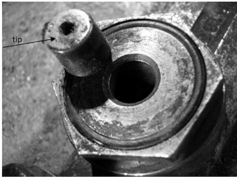
**Figure 2:** Drawing die (matrix) with a tip (pressure type)
