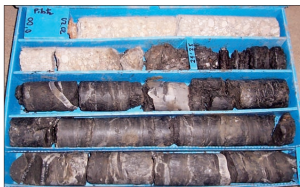
Fig. 15: Inspection samples of the endpoints of 1,000 mm diameter piles which confirm the presence of folded gypsum without signs of karstification.
