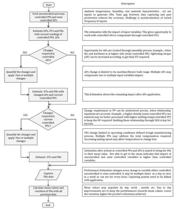
Fig. 6 Monitoring system application flow
