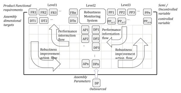
Fig. 5 A schematic representation of the robustness monitoring system connecting PPs and FRs
