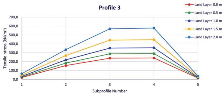
Figure 10. Different soil layer (on the top of the cliff, Fig. 3) height and cliff critical profile tensile stresses (profiles 3-1 to 3-5).
