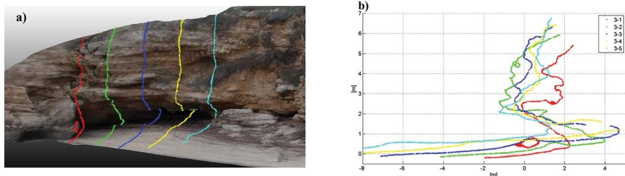
**Figure 9.** Cliff profiles (3–1 to 3–5 with an offset of 2m between each other) parallel to profile 3: a) 3D point cloud; b) 2D profiles delivered from 3D point cloud.
