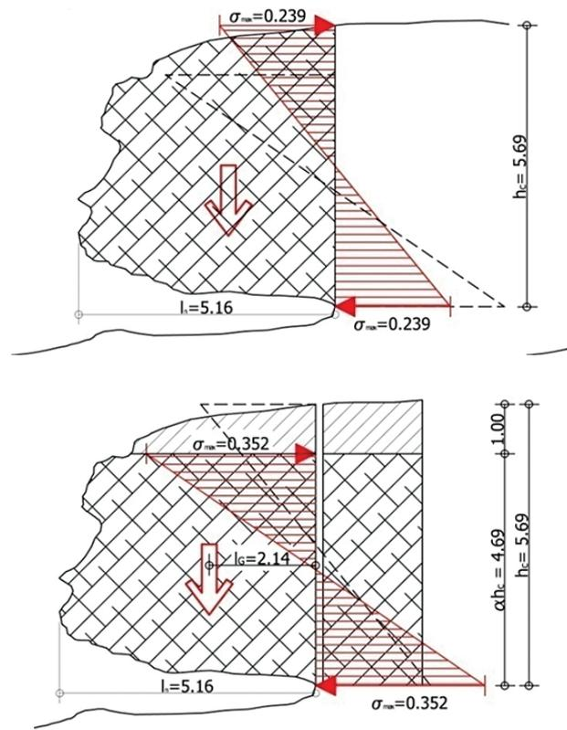
**Figure 8.** Stress distribution inside a cliff (profile 3) with no tension crack (a) and with a tension crack – soil layer (b), and the main variables used in the calculation.
