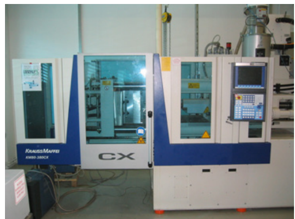
Fig. 1. The used injection molding machine KraussMaffei KM 80 CX-SP for experimental trials
