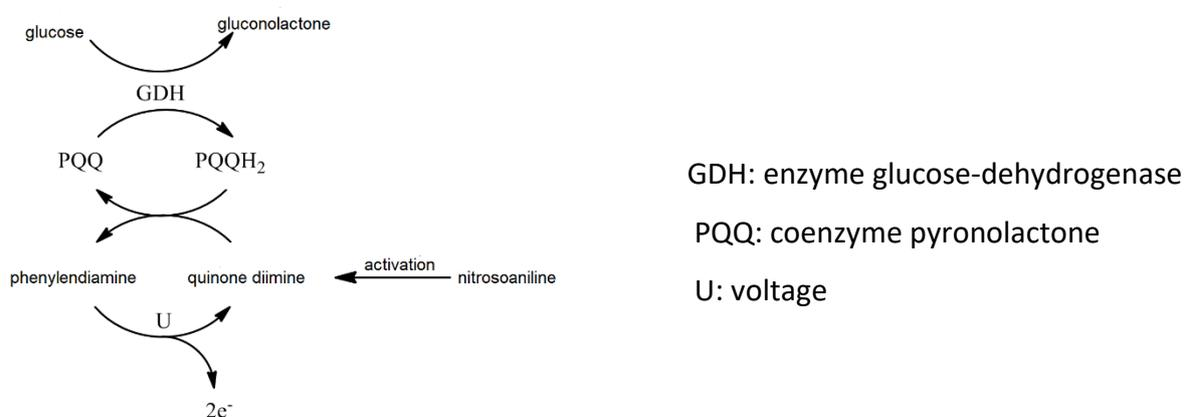
**Figure 3.** Electrochemical reaction in glucometer Accu-Check® Guide.
