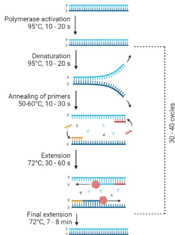
**Figure 3.** PCR principle and phases. Created with biorender.com.
