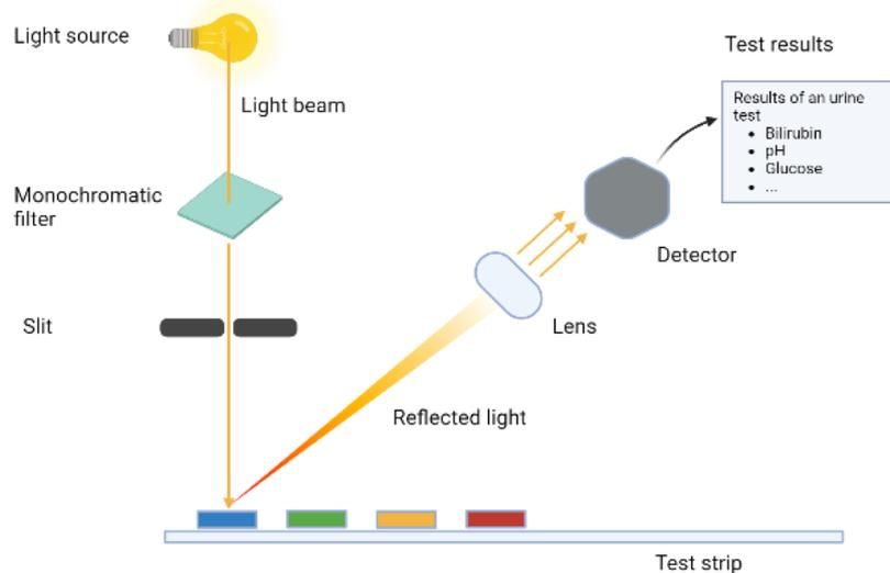
**Figure 2.** Schematic representation of reflectometer. Created with BioRender.com
