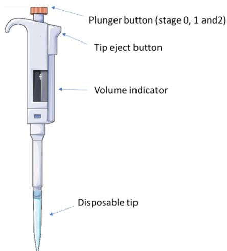
**Figure 2.** Schematic representation of the pipette. The scheme was prepared using SMART - Servier Medical ART 3000.
