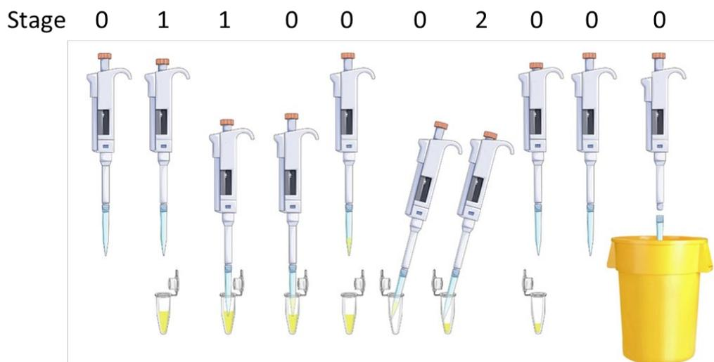
**Figure 3.** Schematic representation of the pipetting procedure. The scheme was prepared using SMART - Servier Medical ART 3000.
