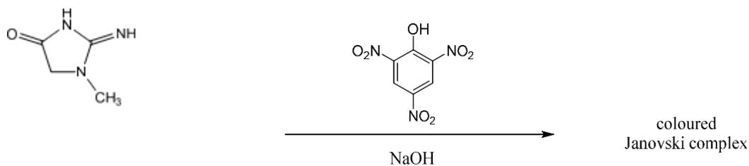
**Figure 1:** Schematic representation of Jaffe reaction.
