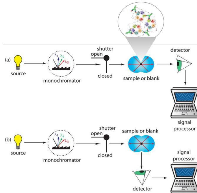
**Figure 2.** The light path and the detection of scattering by turbidimetry (a) and nephelometry (b).
