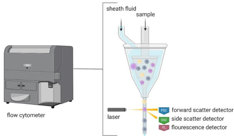
**Figure 1.** Drops of injected sample migrate from injector towards narrow and strong current of the sheath fluid. The precise control of the velocity of both currents enables the alignment of cells, which then individually pass the source of light. Created with BioRender.com
