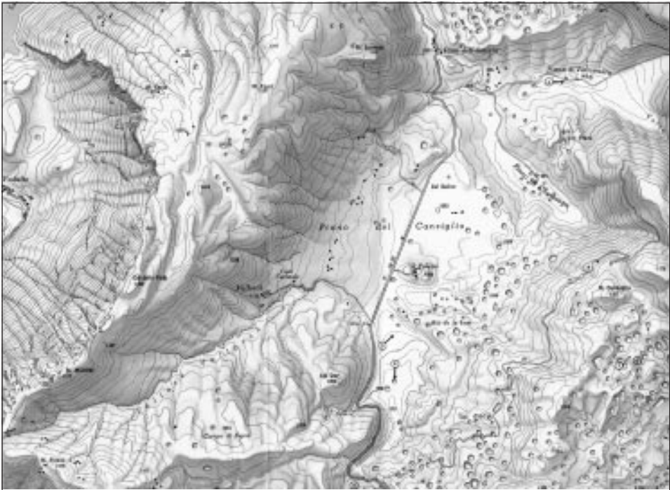
Fig. 10: Map of the Piano del Cansiglio polje basin in the Cansiglio-Cavallo mountain group (after Castiglioni, 1960). The western side and part of the bottom of the basin are formed by the feebly karstifiable marly limestone called "Scaglia Cinerea", while most of the bottom, the western slope and the plateaus encircling the basin are mainly in reef limestones of early and middle Cretaceous (Calcare di Monte Cavallo). Consequently Lehmann described this inactive polje as a "Gesteingrenzenpolje" (polje of lithological contact, a kind of "borderpolje").
