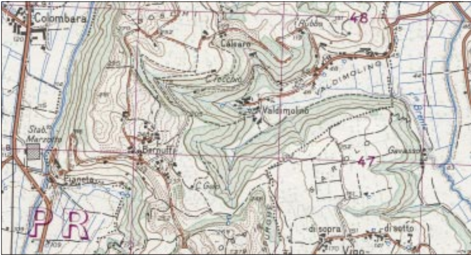
Fig. 12: The aquifer in the alluvial deposit of the bottom of Valdagnò (left side) loses water across the ridge feeding the karst spring of the pocket valley of Valdimolino a tributary of Val d'Onte (right side) (Lessini Mt.) (the sides of the squares correspond to 1 km; the sector is part of the Topographical Map of Italy at the scale 1:25.000, 49 I SE, Arzignano, of the Italian Military Geographical Institute).
