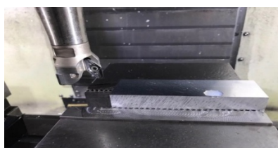
Fig. 3 Experimental realization – clamping of the blank
