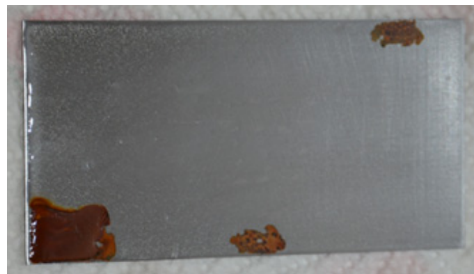
Fig. 8 Test of corrosion in the open air for EMIM-EtSO 4 after 4 days
