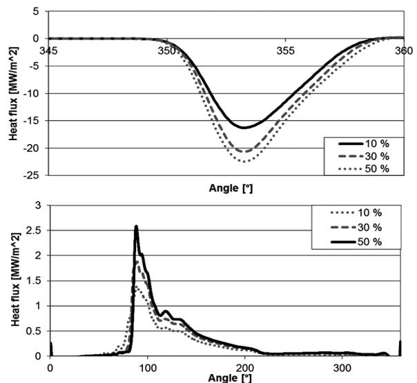
**Figure 3:** Influence of the slab reductions on the heat flux computed from the thermocouple situated 0.8 mm under the roll surface. The contact with the hot strip is on the top and the cooling of the roll is on the bottom.
