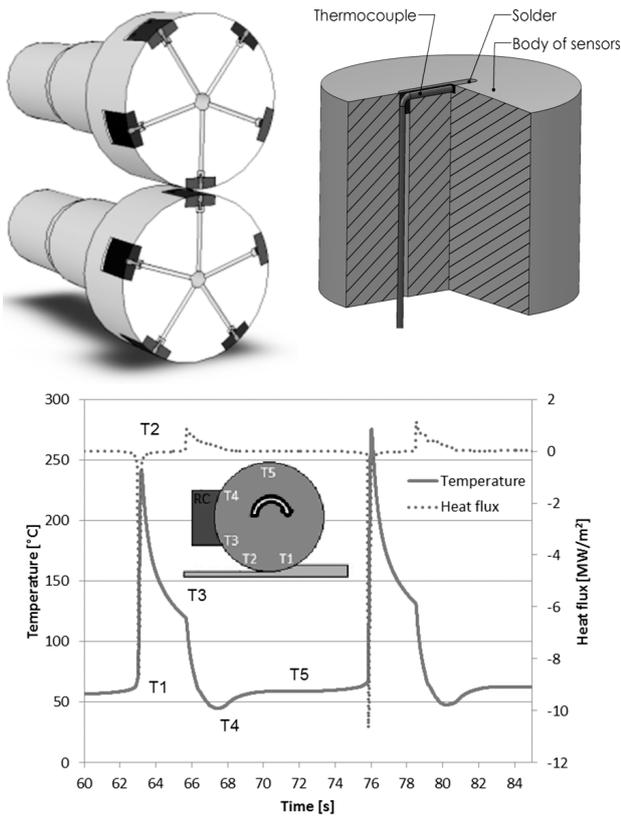
**Figure 1:** Cross-section of the rolls with the inserts from HiCr and HSS materials and the holes for the thermocouple wires; a detail of the plug with a soldered shielded thermocouple; temperature data of the two roll cycles (depth of 0.4 mm, speed of 0.1 m/s, reduction of 10 %) **Slika 1:** Prečni prerez valja z vložki iz materialov HiCr in HSS in luknje za žico termoelementov; podatki o temperaturah pri dveh ciklih valjanja (globina 0,4 mm, hitrost 0,1 m/s, odzvem 10-odstoten)
