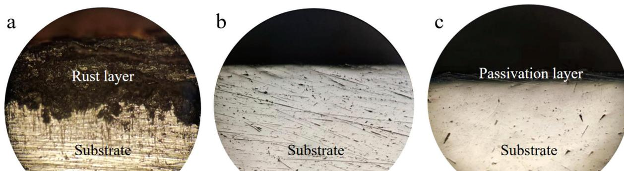
Figure 7: Analysis of microscopic morphological changes at the fracture: a) before pickling, b) after pickling, c) after passivation
