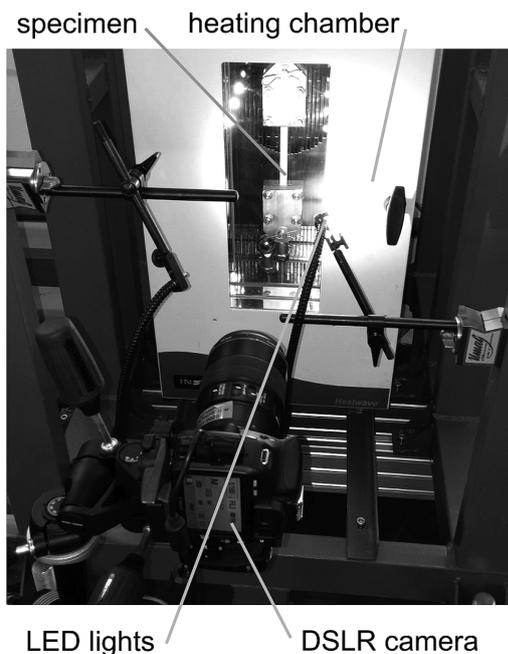
**Figure 4:** Image of the experimental setup and a specimen mounted in the thermal chamber
