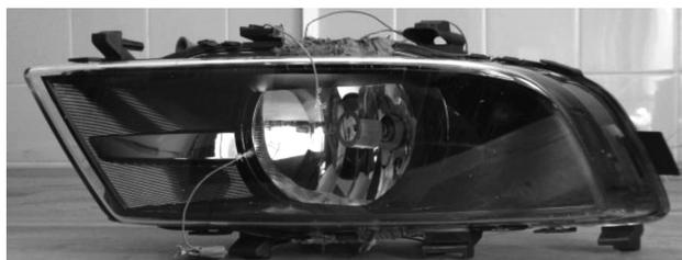
**Figure 1:** Lamp with thermocouples, front view
