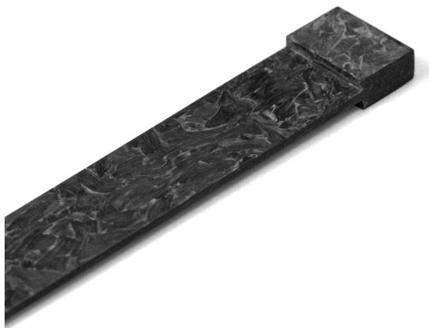
**Figure 1:** Image of a C/PPS sheet used to prepare a specimen
