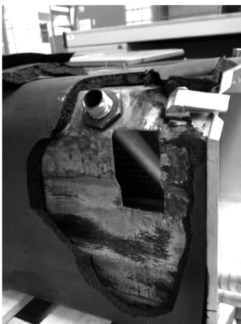
**Figure 1:** Corroded outer surface below the insulation
