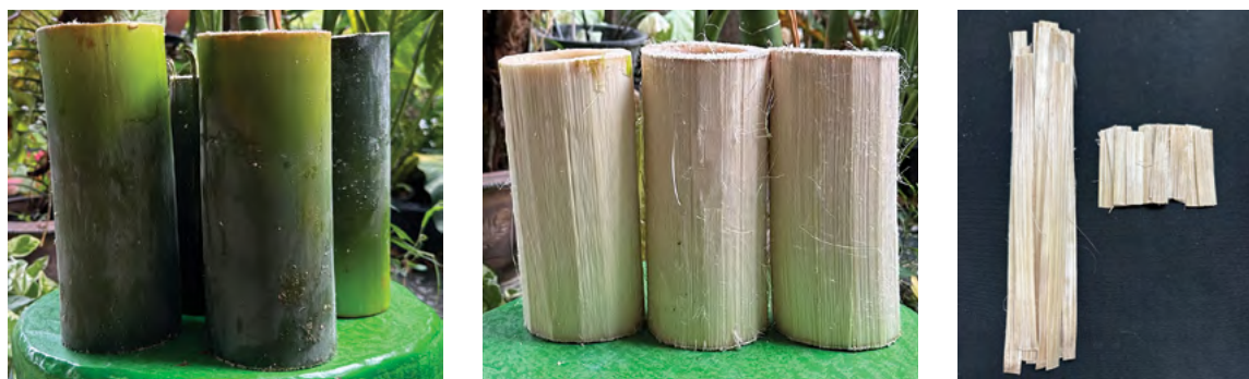
Figure 1: Splitting bamboo into strips (raw material for the boiling process)
