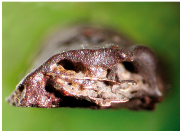
Fig. 5: Fragment of the 3 rd front bridge, transverse fracture (cf. fig. 1: A ); width ca 3.5 mm, height ca 1.5 mm. Three layers of bronze are visible in the iron. Not to scale (photo: S. Perovšek).
