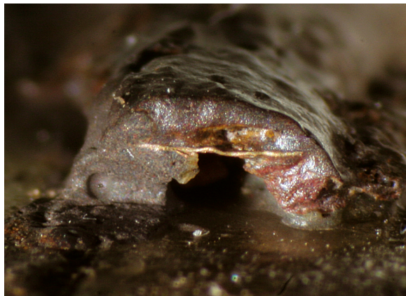
Fig. 6: Fracture of the fragment of the 3 rd front bridge still attached to the scabbard (cf. fig. 1: B ); width of the fracture ca 3.6 mm, height 1.4 mm. A layer of bronze is visible in the iron. Not to scale (photo: S. Perovšek).
