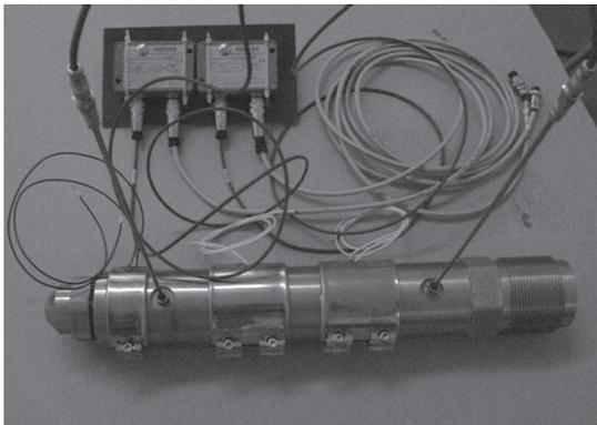
Fig. 1. Nozzle with sensors for 3000T Machine
