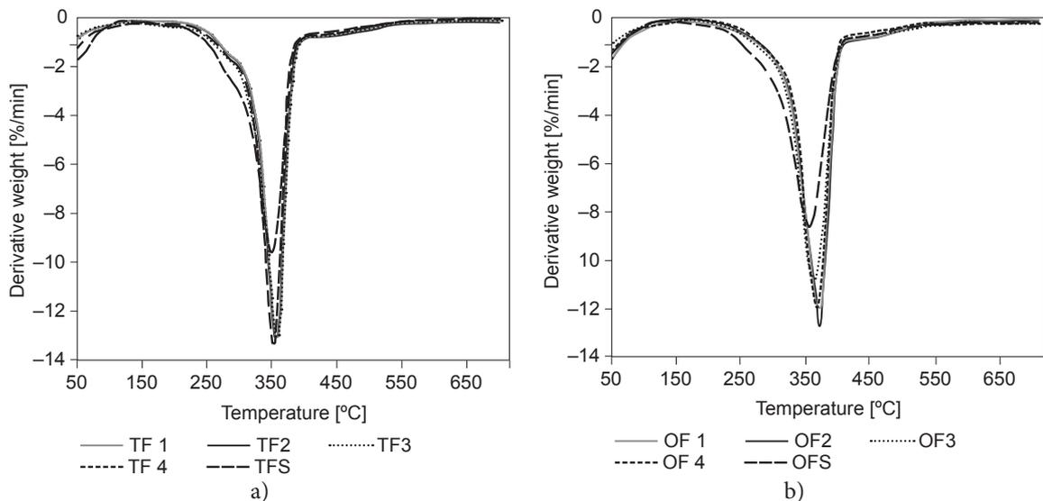
Figure 12: Comparison of DTG curves of: a) textile flax fibres separated into four length groups (TF1-TF4) and shives (TFS); b) oleaginous flax fibres separated into four length groups (OF1-OF4) and shives (OFS)
