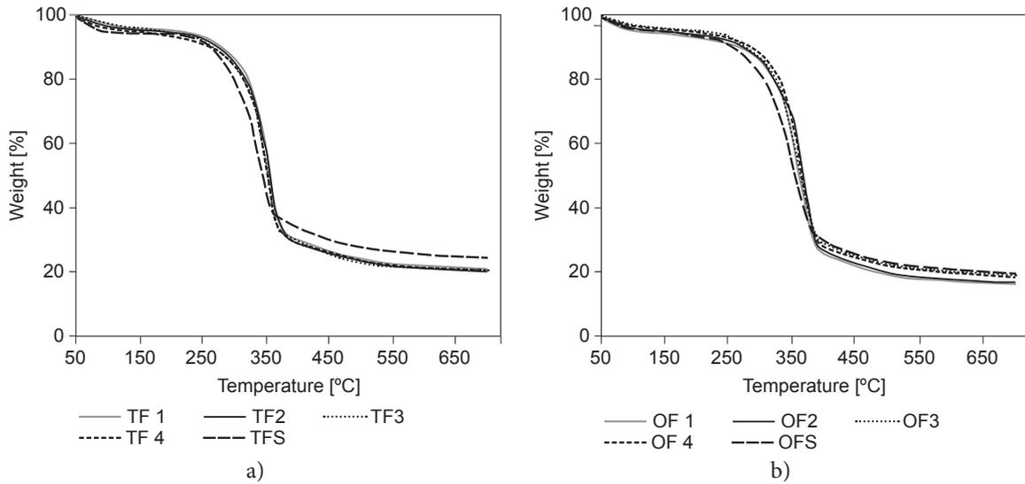
Figure 11: Comparison of TGA curves of: a) textile flax fibres separated into four length groups (TF1-TF4) and shives (TFS); b) oleaginous flax fibres separated into four length groups (OF1-OF4) and shives (OFS)
