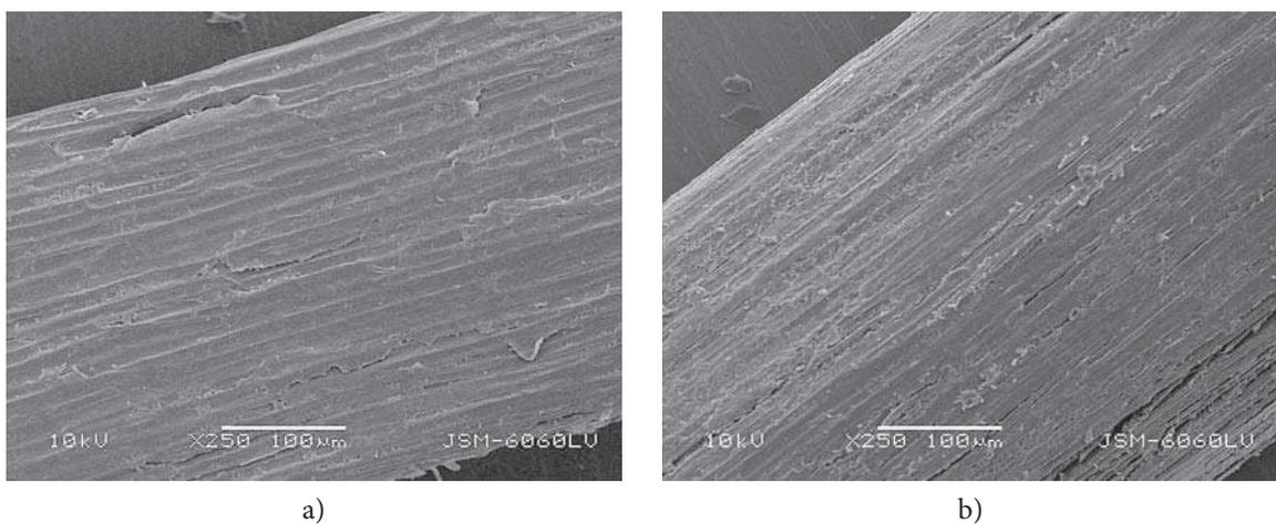
Figure 5: SEM micrographs of shives: longitudinal views (magnification 250×) of textile (a) and oleaginous flax (b)
