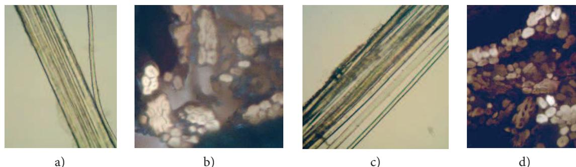
Figure 3: Optical microscopy images of flax fibres: longitudinal views (magnification 100 $\times$ ) and cross-sectional views (magnification 200 $\times$ ) of textile flax fibres (a, b) and oleaginous flax fibres (c, d)
