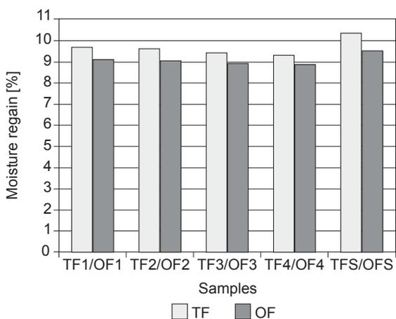
Figure 6: Moisture regain of flax fibrous material – technical fibres of textile flax separated into four length groups (TF1–TF4) and shives (TFS); and technical fibres of oleaginous flax separated into four length groups (OF1–OF4) and shives (OFS)
