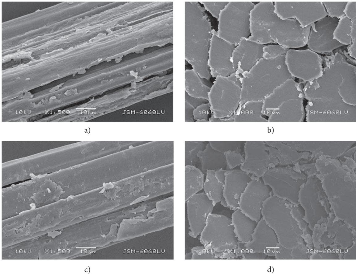
Figure 4: SEM micrographs of flax fibres: longitudinal views (magnification 1500×) and cross-sectional views (magnification 1000×) of textile (a, b) and oleaginous flax fibres (c, d)
