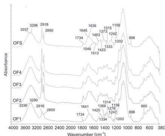
Figure 10: FT-IR spectra of oleaginous flax fibres separated into four length groups (OF1–OF4) and shives (OFS)
