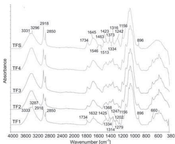
Figure 9: FT-IR spectra of textile flax fibres separated into four length groups (TF1–TF4) and shives (TFS)
