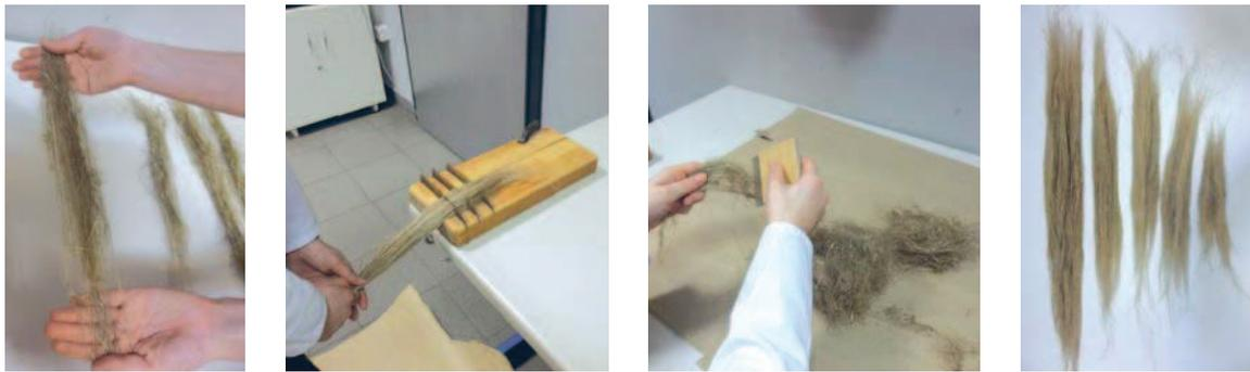
Figure 2: Cleaning, orientation and combing of oleaginous flax technical fibres
