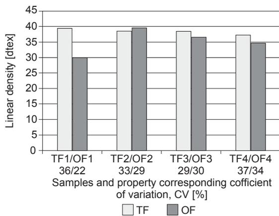
Figure 8: Average linear density of flax technical fibres separated into four length groups – textile flax (TF1–TF4) and oleaginous flax (OF1–OF4)
