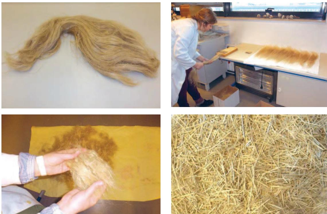
Figure 1: Cleaning, orientation and combing of textile flax technical fibres, and separated shives
