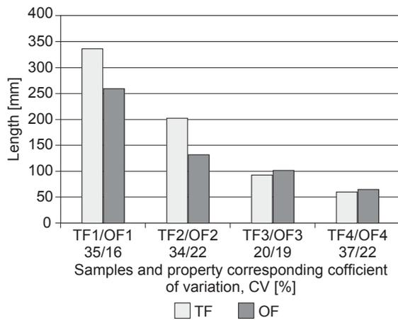
Figure 7: Average length of flax technical fibres separated into four length groups – textile flax (TF1–TF4) and oleaginous flax (OF1–OF4)
