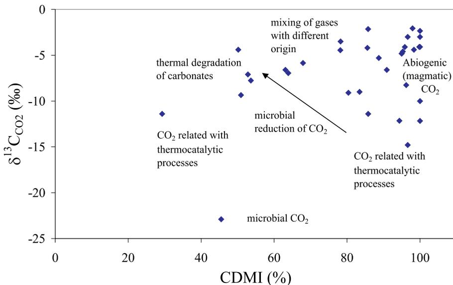
**Figure 4.** Interpretation of the origin of CO<sub>2</sub> in the Velenje basin using  $\delta^{13}\text{C}_{\text{CO}_2}$  versus CDMI index in the lignite seam ahead of the working face
