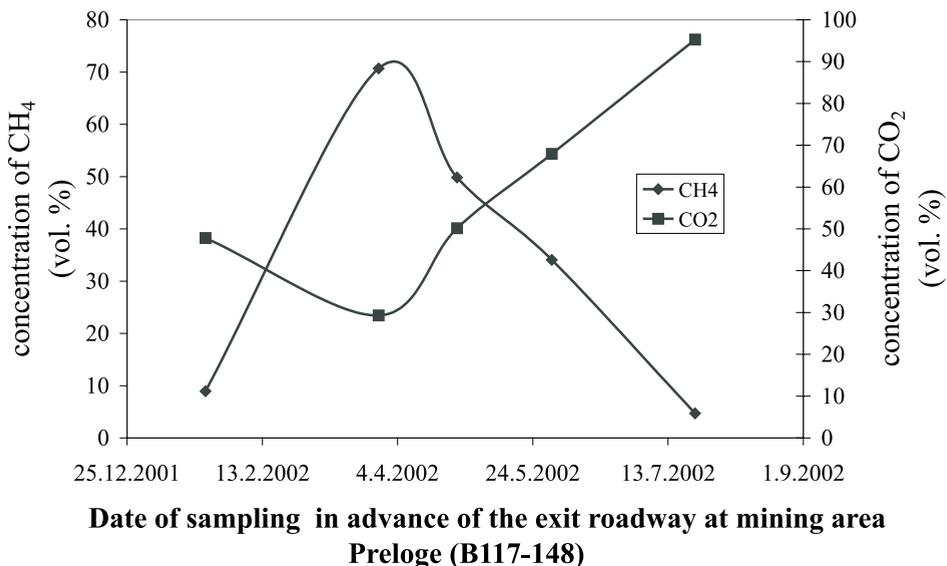
**Figure 2 a.** Concentration of methane versus date of sampling in advance of the exit roadway in the Preloge mining area (B117 – 148) ahead of the working face
