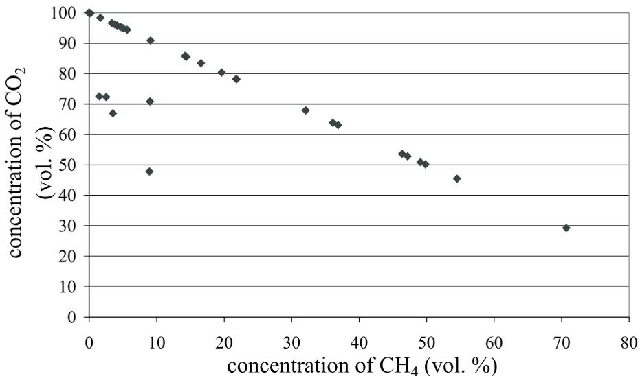
**Figure 2.** Concentration of CO<sub>2</sub> versus concentration of methane in the lignite seam ahead of the working face in the Velenje basin
