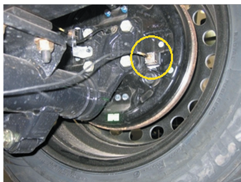
Fig. 11. Accelerometers mounted on the backing plate
