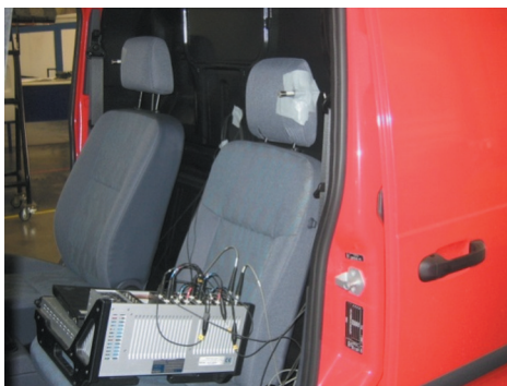
Fig. 10. Microphone positioning in cabin onto driver head guard
