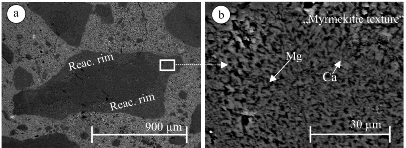
Figure 2: Process of dedolomitisation in sample 2 (after 6 m)
