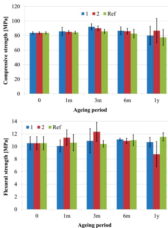
Figure 8: Strength of the mortar bars: a) compressive strength, b) flexural strength
