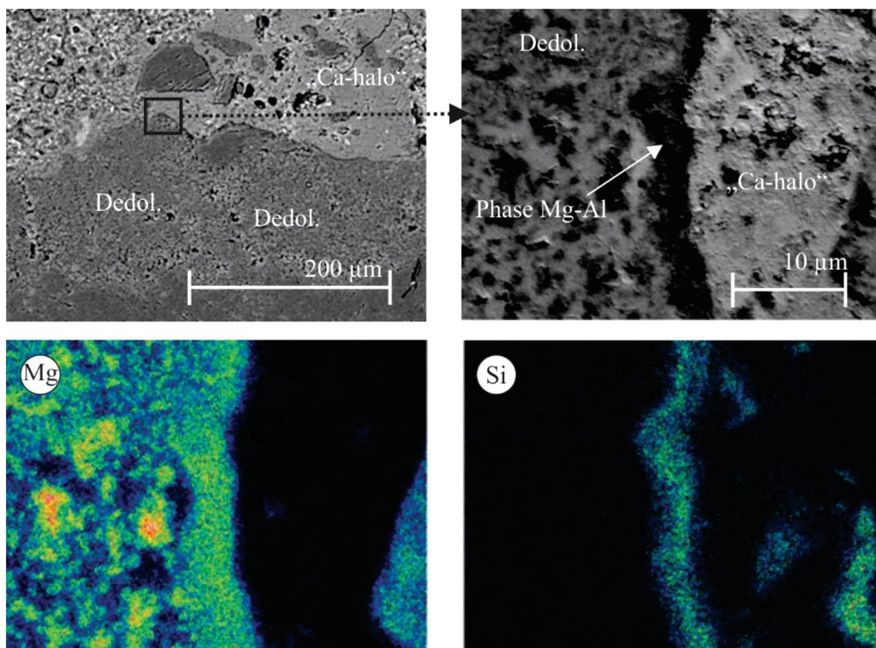
Figure 5: Formation of Mg-Si phase in sample 2 (after 6 m)
