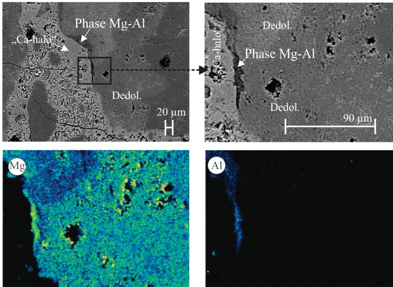
**Figure 4:** Formation of Mg-Al phase in sample 2 (after 3 m)
