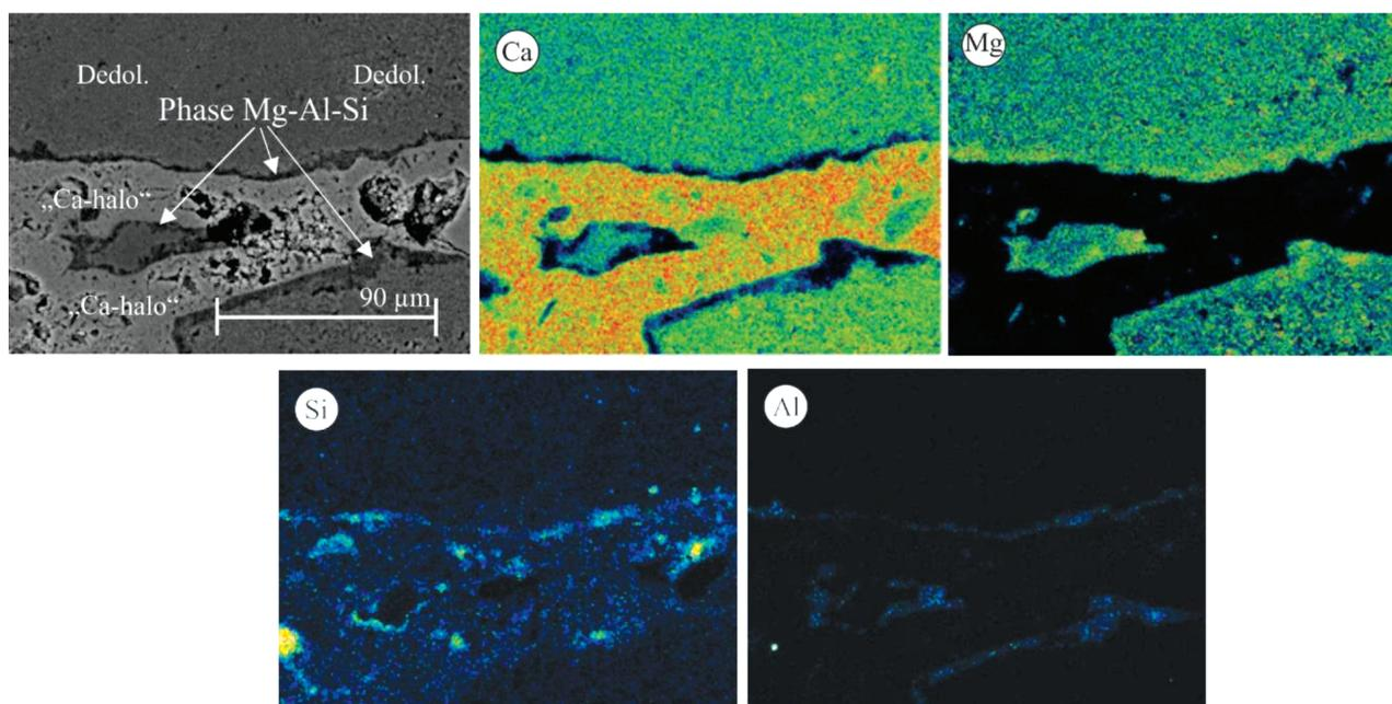
Figure 6: Formation of Mg-Si-Al phase in sample 2 (after 1 y)
