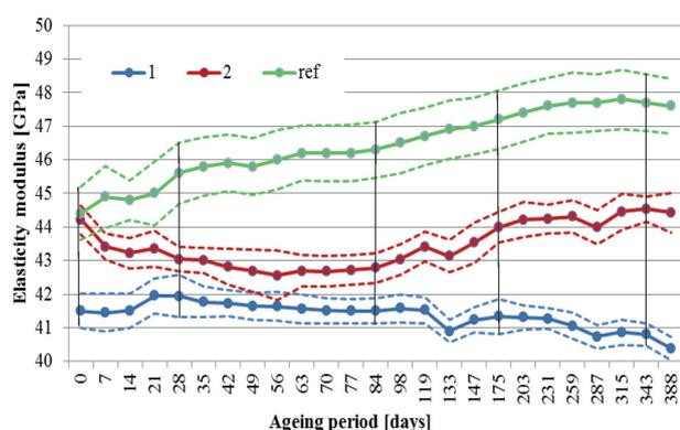
**Figure 9:** Changes in elasticity modulus of samples 1 and 2, compared to samples in water at 20 °C
