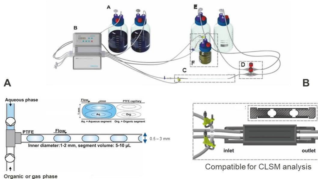
Figure 1: Schematic of the capillary biofilm reactor (CBR). *Top*: Overall system with medium reservoir (A), pump (B), cultivation chamber (C), sampling port (D), and waste (E). Alternative feeding option (F). *Below A*: Concept of a capillary reactor run in segmented flow fashion. *Below B*: Flow cell for confocal laser scanning microscopy adapted to CBR geometries. Figure modified from<sup>1</sup>.
