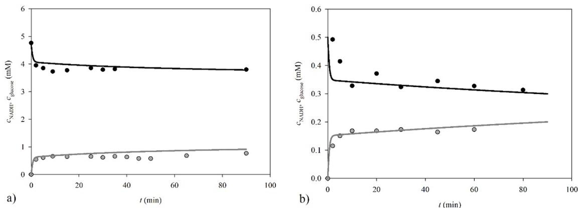
Figure 1: Biocatalytic glucose oxidation by GDH in the batch reactor ( $\gamma_{\text{GDH}} = 0.002 \text{ mg/ml}$ ;  $0.1 \text{ mM}$  TRIS-HCl buffer pH 7;  $T = 40 \text{ }^\circ\text{C}$ ;  $V_{\text{reactor}} = 50 \text{ ml}$ ) at different initial substrate concentrations: a)  $c_{\text{glucose}} = 4.7 \text{ mM}$ ,  $c_{\text{NAD}^+} = 1.1 \text{ mM}$  and b)  $c_{\text{glucose}} = 0.5 \text{ mM}$ ,  $c_{\text{NAD}^+} = 1.1 \text{ mM}$ ; ( $\bullet$ ) glucose, ( $\circ$ ) NADH, (—) model
