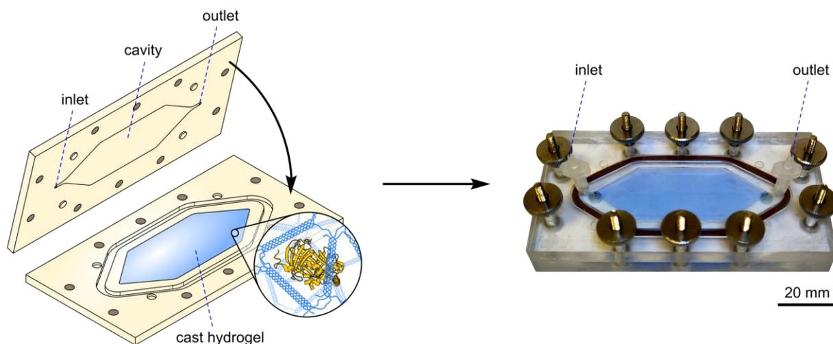
Figure 1: Assembly of the flat-bed agarose reactor for the investigation of enzyme leaching.
