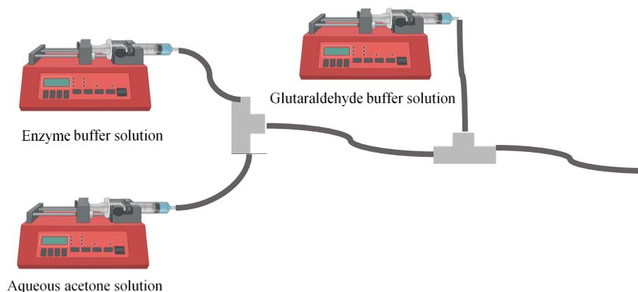
Figure 2: Scheme of a continuous CLEA-HRP production
