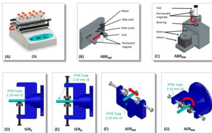
Figure 1: Modes of the reactors for the MNPs-catalyzed biotransformations
