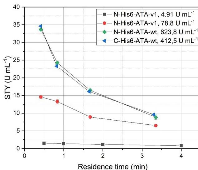
Figure 2: Space time yields (STY) obtained in the microreactor with Tiss®-IMAC-Cu using various enzymes and enzyme loads as specified in the legend. The biotransformations were performed at 30°C with 40 mM (S)- $\alpha$ -MBA and PYR in 20 mM phosphate buffer, pH 8, without added PLP.
