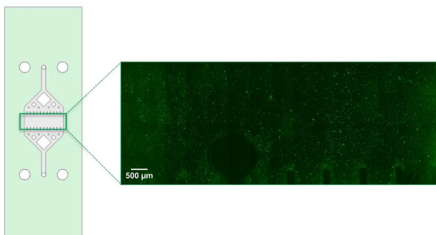
Figure 1: Microfluidic device workflow outlining a homogeneous GFP expression throughout the chamber upon lentiviral transduction of a suspension cell line.
