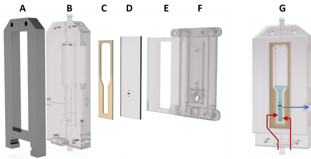
**Figure 1:** 3D-printed micro bubble column reactor (MBCR) setup, exploded-view: (A) Connector clip, (B) 3D-printed MBCR, (C) sealing, (D) sensor slide, (E) frame for sensor slide, (F) docking station, (G) assembled MBCR with sensor slide and micro channels for sampling (blue), as well as substrate/media inlets (red).
