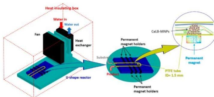
Figure 2: Schematic illustration of the U-shape reactor
