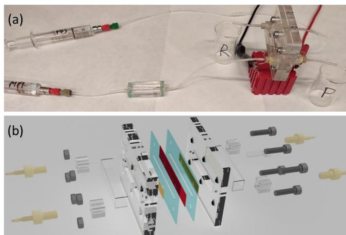
Figure 1: (a) Photo of the modular system for the synthesis of mandelic acid enantiomers; (b) Detail scheme of the membrane separator.
