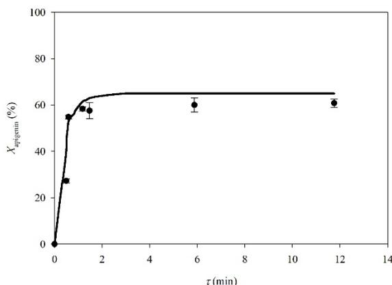
Figure 2: Influence of residence time on apigenin conversion for experiment performed in a microreactor (● experimental results, — mathematical model)
