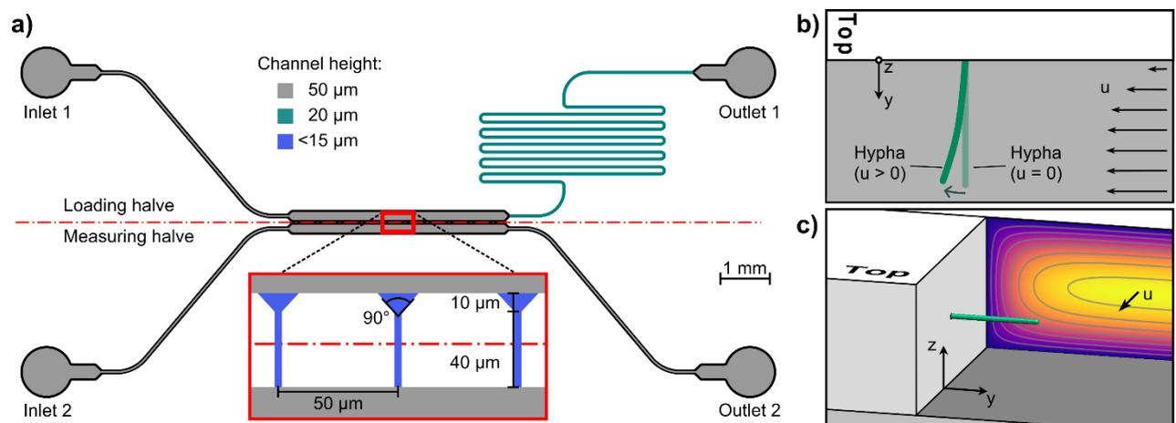
Figure 1: a) Schematic view of microfluidic system design with zoomed in view of the growth channels. Schematic top view (b) and perspective view (c) of the measurement configuration in the measurement chamber (system cover plate not shown). In b) the light and dark green shapes resembles the initial and deflected hyphal shape. The flow velocity is indicated as  $u$ .
