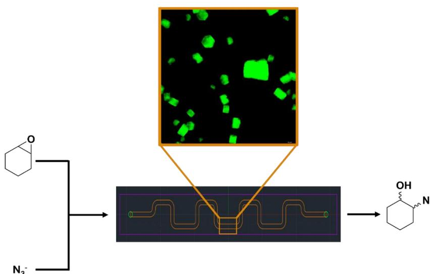
Figure 1: HheG D114C CLECs (stained with fluorescein isothiocyanate) on a glass microchip catalyzing the ring opening of cyclohexene oxide with azide as a model reaction.
