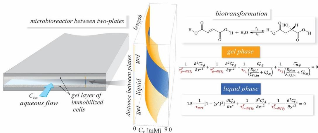
Figure 1: Presentation of L-malic acid production in microreactor between two layers of immobilized yeast cells.<sup>3</sup>
