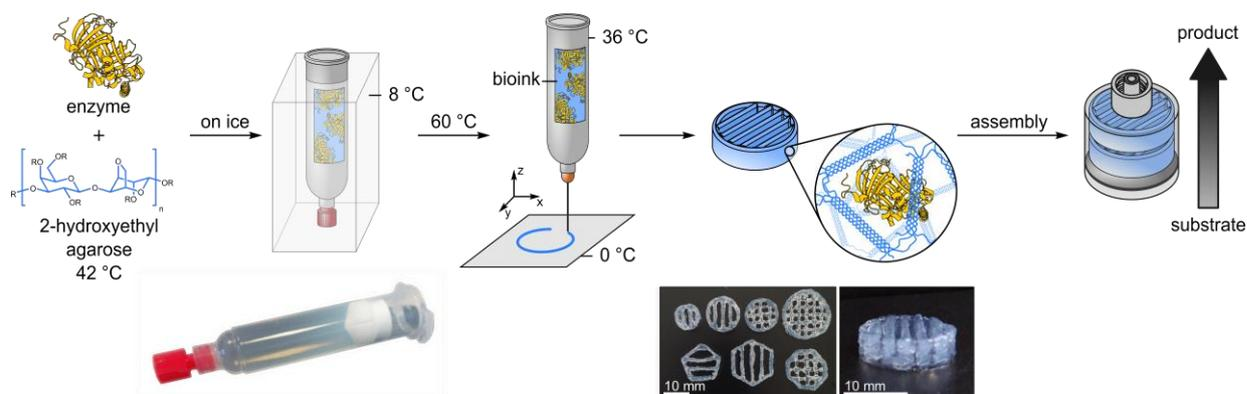
Figure 1: Additive manufacturing process for entrapment of enzymes in 3D printed hydrogel structures.
