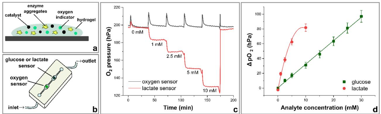
Figure 1: a) composition of the sensor spots; b) placement of the spots in a microfluidic cell used for the sensors' characterization; c) response of the lactate sensor exposed to the analyte in 0-10 mM concentration range; d) response curves for glucose and lactate sensors with diffusion membrane of 0.5% porosity.
