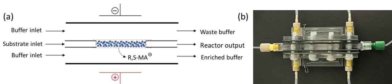
Figure 1: (a) Schema and (b) photo of the fully integrated system for the synthesis of mandelic acid enantiomers.
