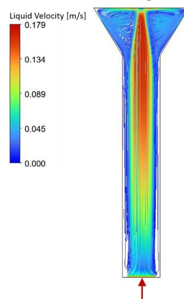
**Figure 2:** Steady-state multiphase model of the MBCR (RANS/Euler-Lagrange-approach), gas inlet (red arrow).
