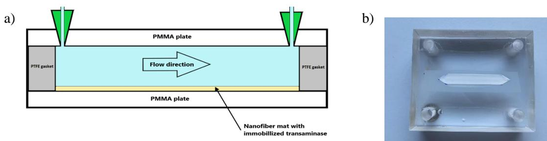
Figure 1: a) A scheme of a microreactor between two plates with an integrated nanofiber mat and b) an open reactor assembly without the PTFE gasket.
