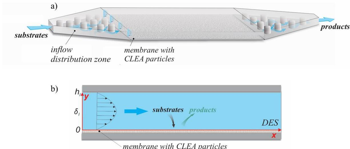
Figure 1: a) scheme of a microreactor between two plates with CLEA-ADH immobilized on the membrane surface; b) physical domains of a 2D mathematical model.
