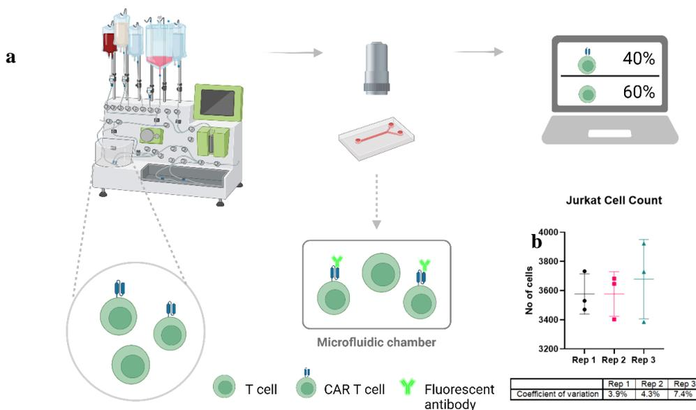
Figure 1: Microfluidic PAT for CAR T cell therapy manufacturing (a) A workflow for microfluidic analytical system integrated with CAR T cell manufacturing technologies such as CliniMACS Prodigy®, aiming to provide quantitative analysis of T cells in process by labelling them with fluorescent antibodies (b) Results from immunofluorescence-based counting of Jurkat cells. This figure was made in Biorender.
