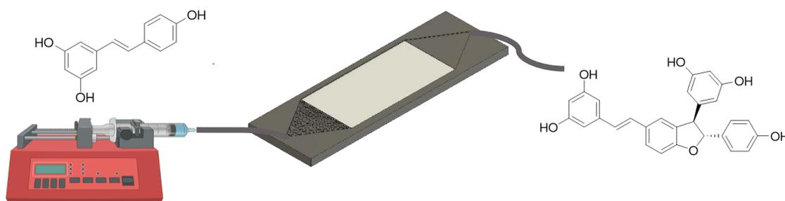
Figure 3: Scheme of a continuous  $\delta$ -viniferin production in a microreactor with CLEA-HRP immobilized on the membrane surface
