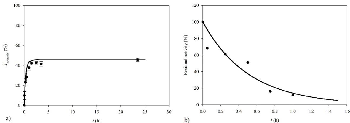
Figure 1: a) Dynamic change of apigenin conversion and b) HRP process stability for experiment performed in a batch reactor (● experimental results, — mathematical model)
