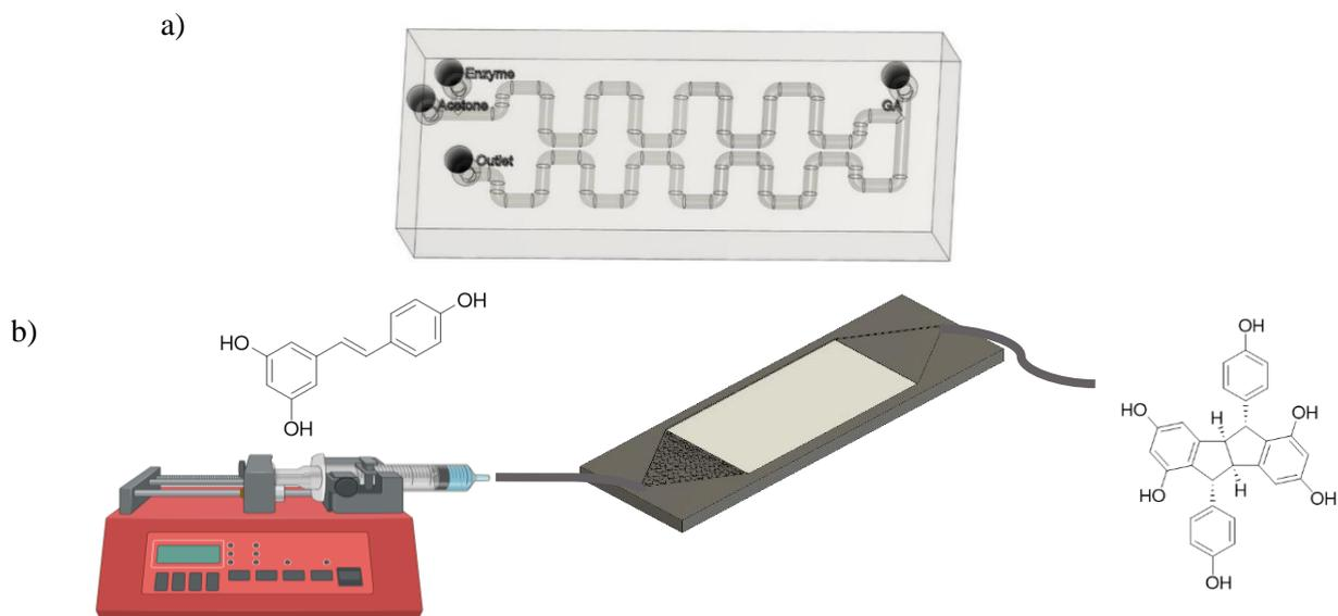
Figure 2: a) 3D-printed microflow system for CLEA-HRP production; b) continuous production of pallidol utilizing immobilized CLEA-HRP on a membrane integrated in a 3D-printed microreactor.
