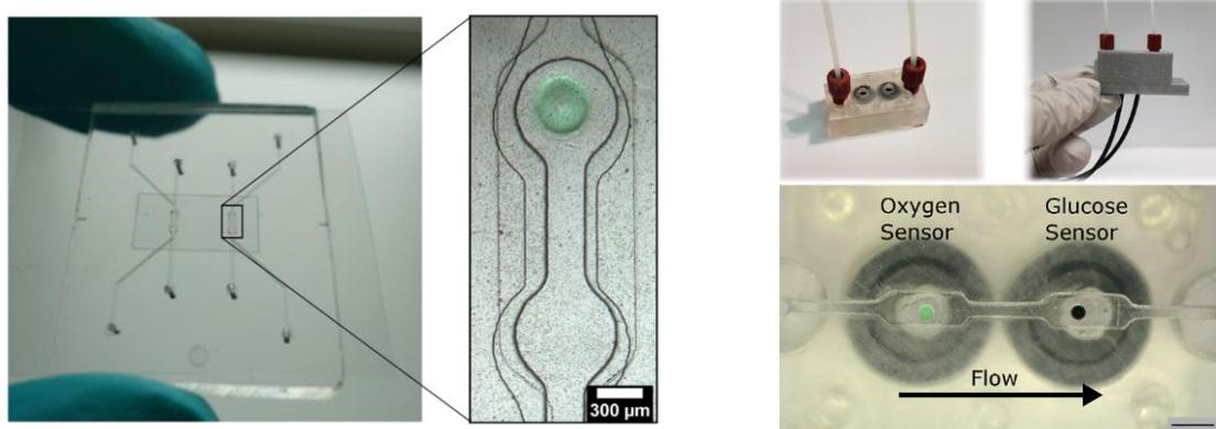
Figure Left: Heart-on-Chip with integrated optical oxygen sensors (green dots). Figure Right: Glucose sensor integrated in a microfluidic flow cell.
