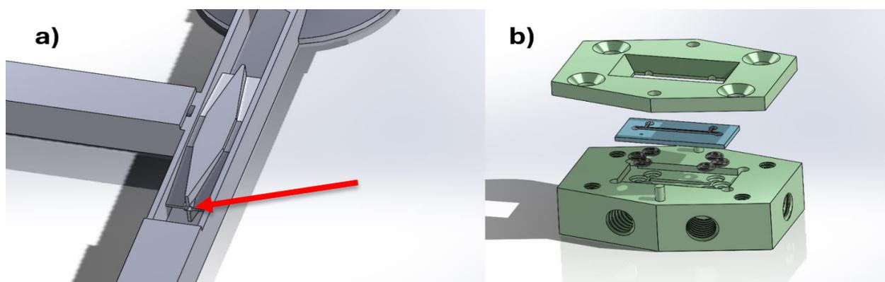
Figure 1: Two renders of the microfluidic device; a) the nozzle designed for the outlet with the same design as the outlet nozzle, and b) a microdevice on a glass substrate (blue) together with the holder (green)
