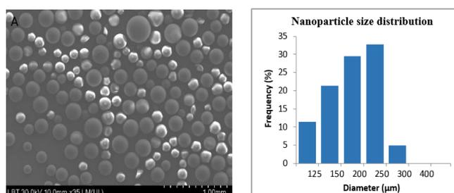
Figure 1: TEM image and nanoparticle size distribution of Immobead T2-150
