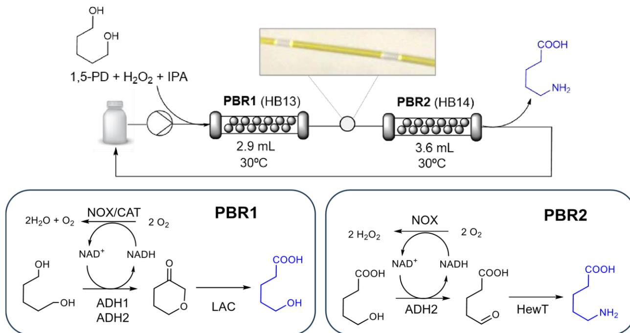
Figure 1: Continuous flow synthesis of 5-AP by telescoped packed-bed reactors.
