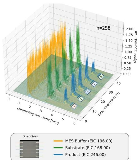
Figure 2: A waterfall diagram of acquired chromatograms of buffer, substrate and product of a model biocatalytic bromination of a run consisting of 5 separate microreactors showcasing the extensive data generation capabilities of this setup.<sup>1</sup>
