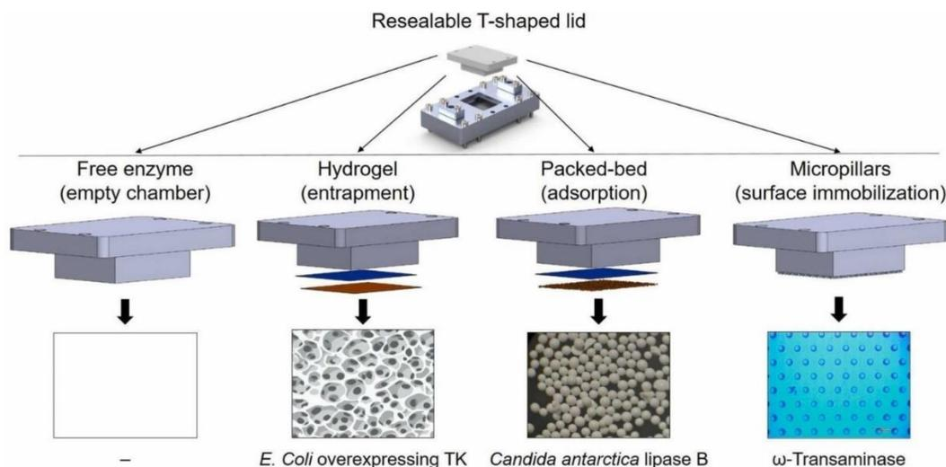
Figure 1: Decoupling application from reactor design for flow biocatalysis applications.
