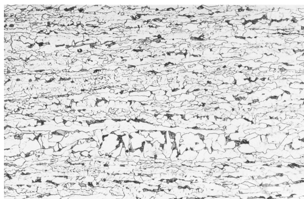
Figure 5: (magn. 200 times) Microstructure of the steel K from Figure 3 rolled in the temperature range from 900 °C to 774 °C
