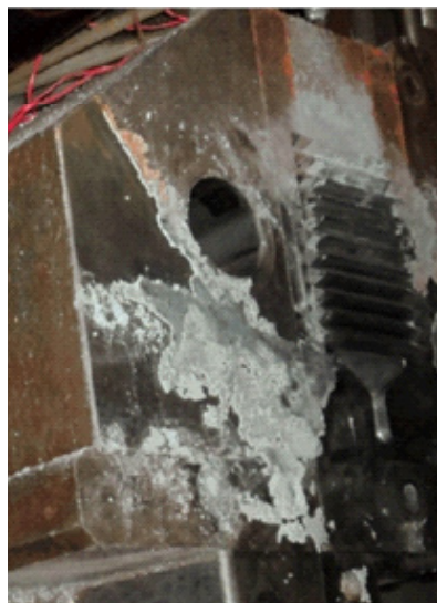
Figure 2: Excessive Flashing seen in Chill Vent
