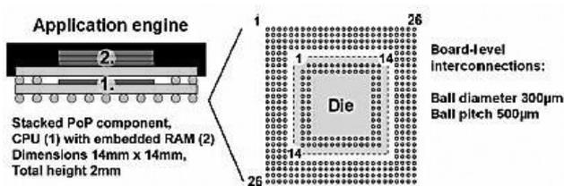
Fig. 11: Application engine component package (Karpinen et al., 2010)
