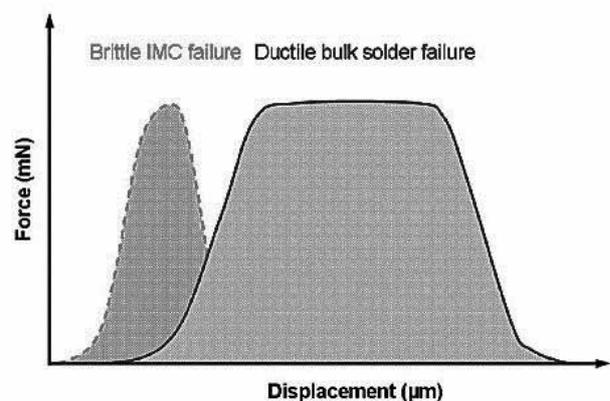
Fig. 5: FBST force vs. displacement (Grafe et al.)
