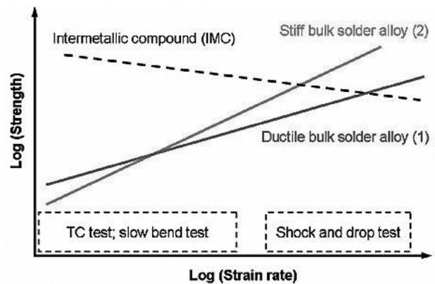
Fig. 4: Joint strength vs. strain rate (Grafe et al.)
