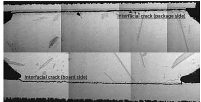
Fig. 1: SAC405 solders joint failure in shock conditions (M.P. Renavikar, 2008)
