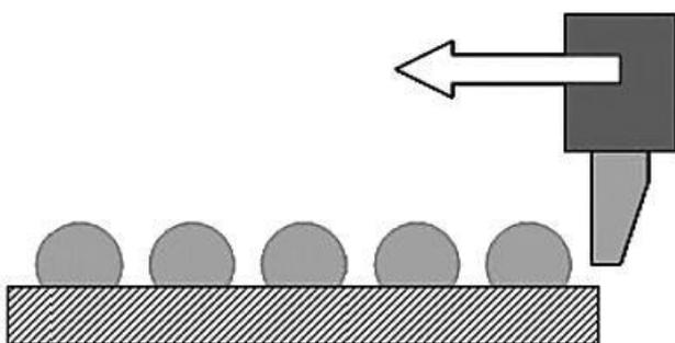
Fig. 3: Fast ball shear test arrangement (Grafe et al.)
