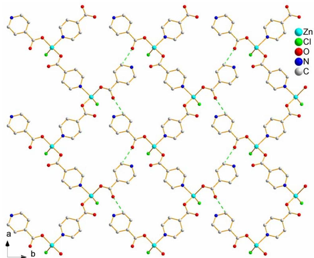
Fig. 2: The 2-D layer formed via the hydrogen bonds in dashed lines: C11-H...O4(-1 + x, 3/2-y, -1/2 + z) 2.938(3) Å, 116.1°.
