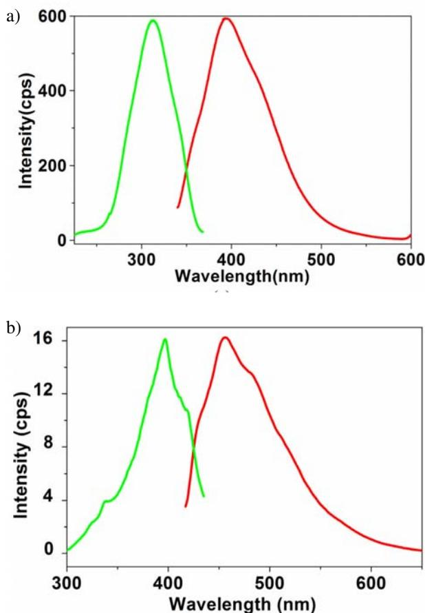
**Fig. 4.** The emission and excitation spectra at room temperature: (a) complex **1** and (b) isonicotinic acid. Red lines: emission spectra; green lines: excitation spectra.
