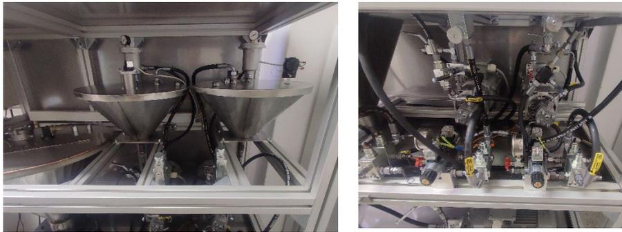
**Figure 1: Conical reservoirs (on the left) to prevent the contaminants to settle down and 4/3-way valves with pressure relief valves for the load of the gear pumps (on the right).**
