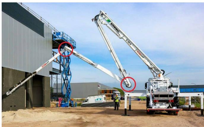
**Figure 1: Concrete Pump Boom with two hydraulic motors.**
