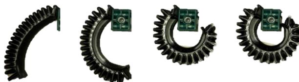
**Figure 16: Pneumatic soft robotic gripper.**
