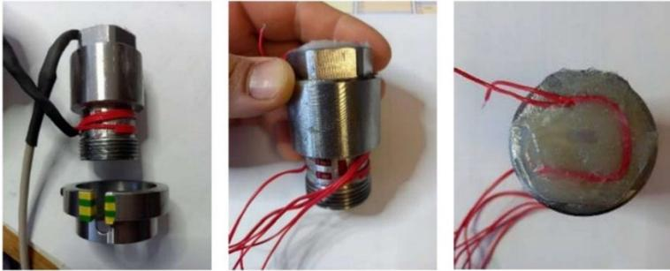
**Figure 9: Modified plug M33x2 equipped with strain gauges**
