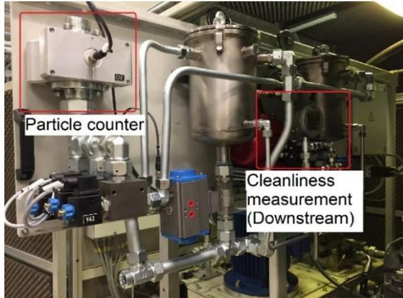
Figure 5: Particle counter and oil cleanliness measurement.
