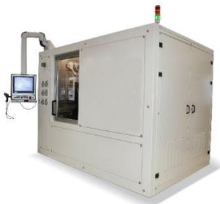
**Figure 1: Test bench for EOL testing**
