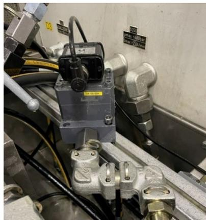
Figure 6: Flow meter mounted on the rail in front side of the test bench.
