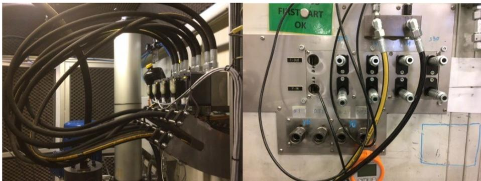
**Figure 4: Additional flow meters which are easily to grab and plug into the tested valve.**
