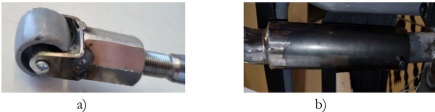
**Figure 2: Made parts for the system operation, a) nut with wheel, b) telescopic rod.**
