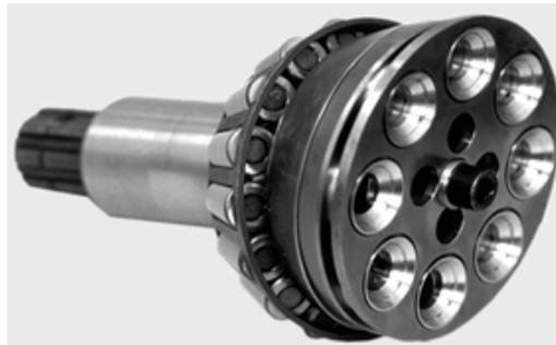
**Figure 2: A detail of drive shaft bearing.**
