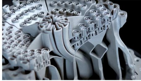
**Figure 14: Hydraulic manifold optimized for efficient flow conditions.**
