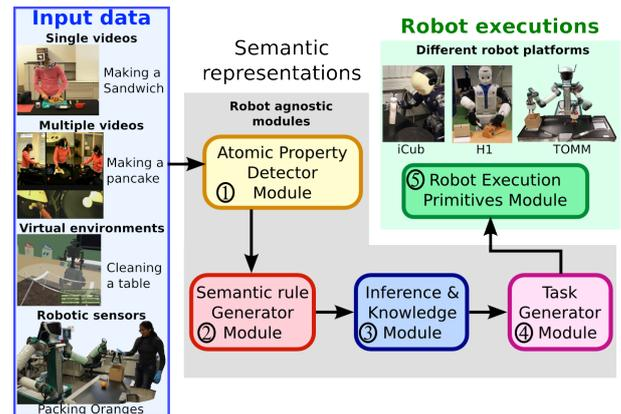
Figure 1: Main modules of our framework for the segmentation and recognition of human everyday activities using multiple sensors.
