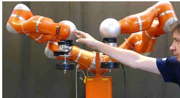
Figure 1: Bimanual robot performing a task while being perturbed by a human.
