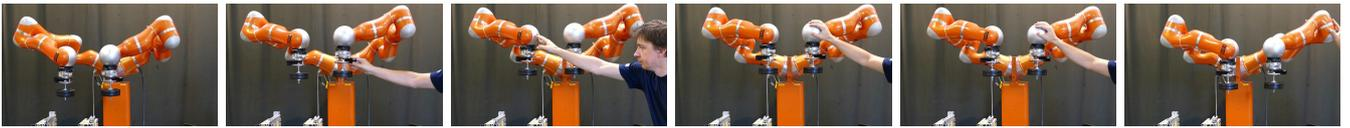
**Figure 4: Bimanual robotic system performing the experimental compliant bimanual task. A person was perturbing the motion.**
