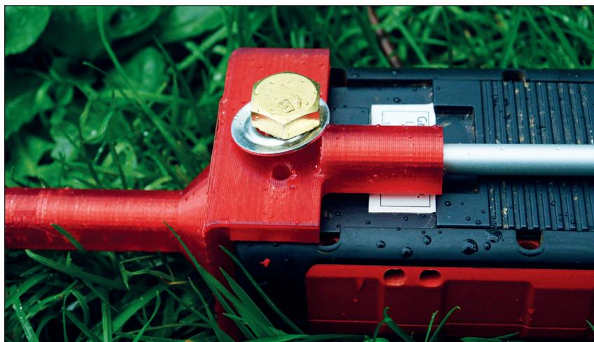
Fig. 2: Attaching the DistoX to the calibration tool with an almost correct bolt. The bolt is slightly too long and we avoided sawing it by adding an aluminum washer. The hole on the tool, which was originally too big, was shrunk using a few layers of nail polish (Photo: M. Perne).
