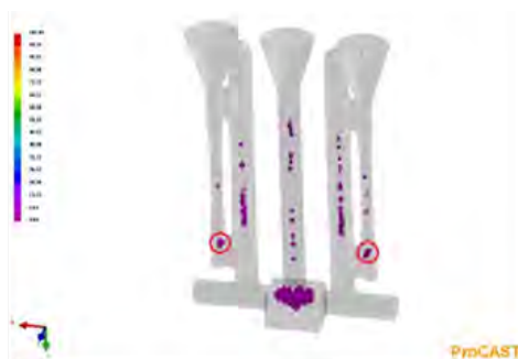
(e) Razmerje poroznosti ulitka / Casting porosity ratio
