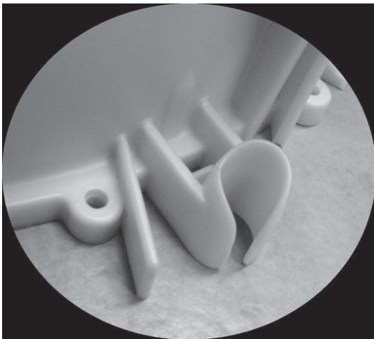
Fig. 4. Short shot at the end of filled cavity
