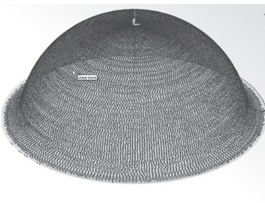
Fig. 10. NC program simulation of toolpath 2
