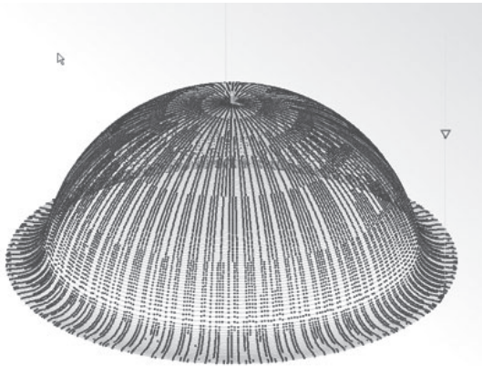
Fig. 12. NC program simulation of toolpath 3
