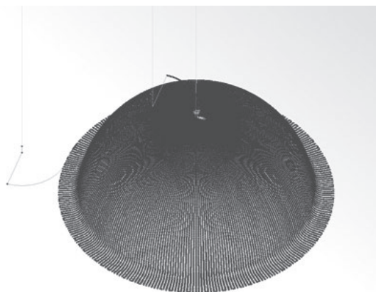
Fig. 14. NC program simulation of toolpath 4
