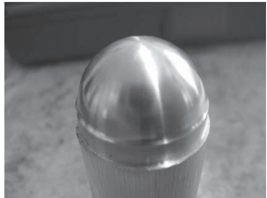
Fig. 19. Finished part after toolpath2
