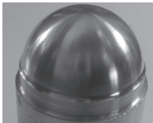
Fig. 23. Finished part after toolpath 4
