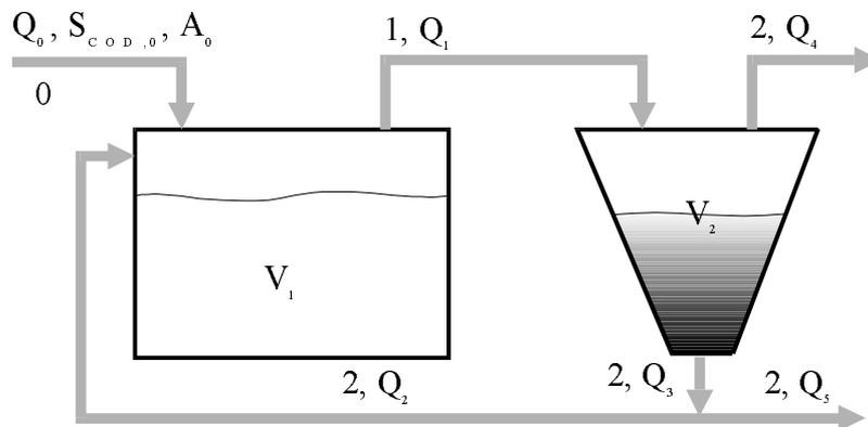
Figure 1. Sketch of the single-stage wastewater treatment plant.
