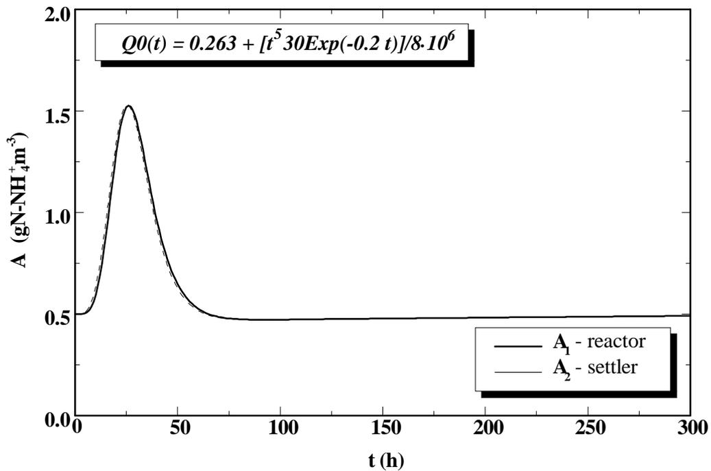
Figure 7. Dynamic response of autotrophs in the reactor and settler at simulation of “real” two-day disturbance of inlet wastewater flow.
