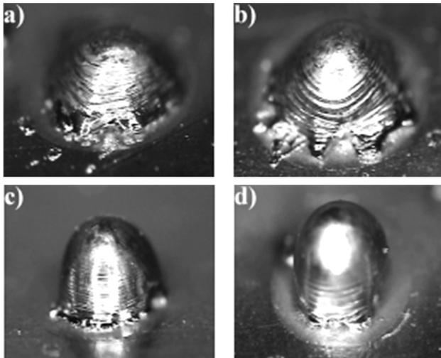
**Figure 10:** Magnifications of typical droplets from the sets produced with different detachment pulses
