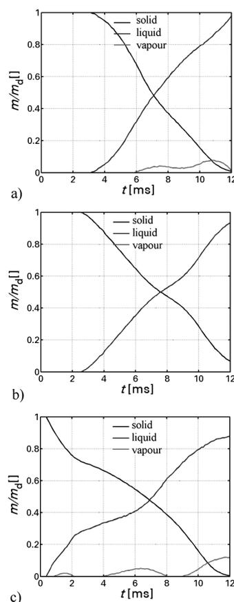
**Figure 4:** Time courses of the shares of the material in solid, liquid and vapour phases during the laser pulses. Graphs correspond to the laser pulses shown in **Figure 3**.
