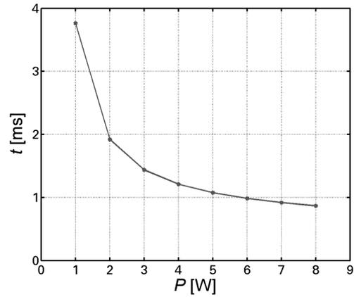
**Figure 8:** Dependence of detachment-pulse duration on the selected laser power
