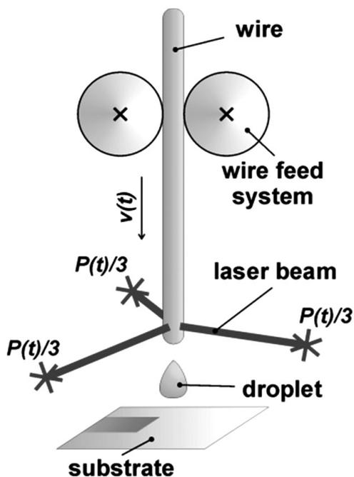
**Figure 1:** In the laser droplet-formation process (LDFP) a thin metal wire is fed to the focus of laser beams. A hot molten droplet is formed at the tip of the wire, detached by a sudden increase in the laser power and deposited on the substrate.
