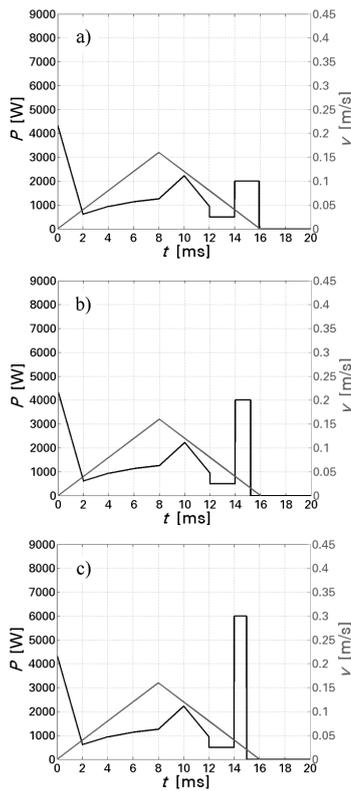
**Figure 7:** Three examples of laser pulses with the same pendant-droplet-formation parts and different detachment parts. Droplet-detachment pulses are of: a) 2000 W, b) 4000 W and c) 6000 W.
