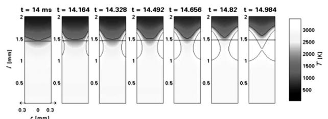
**Figure 9:** Time development of the temperature field during a droplet-detachment pulse
