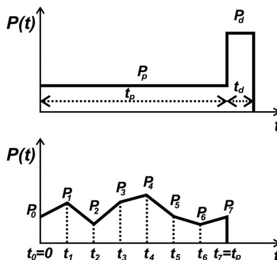
**Figure 2:** Simple laser pulse for LDFP consists of two parts: pendant-droplet-formation part and detachment part (top). In the present work we parameterized the first part of the pulse with seven parameters in order to further optimize the heat input (bottom).
