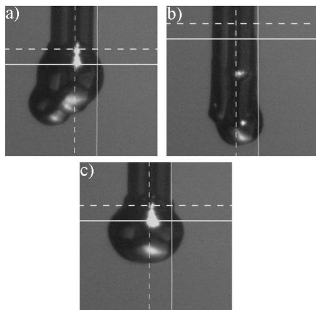
**Figure 6:** Typical examples of experimental outcomes of pendant-droplet formation. Droplets correspond to the laser pulses shown in **Figure 3** denoted with the same letters.
