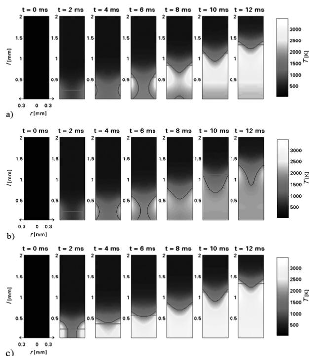
**Figure 5:** Evolution of the temperature field of the wire. Images correspond to the laser pulses shown in **Figure 3**.
