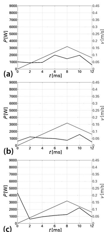
**Figure 3:** Examples of laser pulses (black line): a) laser pulse determined with the fitness function  $J_1$  and laser pulses determined with the fitness function  $J_2$  with the selected final temperatures: b)  $T_{z1} = 2000$  K and c)  $T_{z2} = 3000$  K. Grey line denotes the velocity profile of the wire movement.
