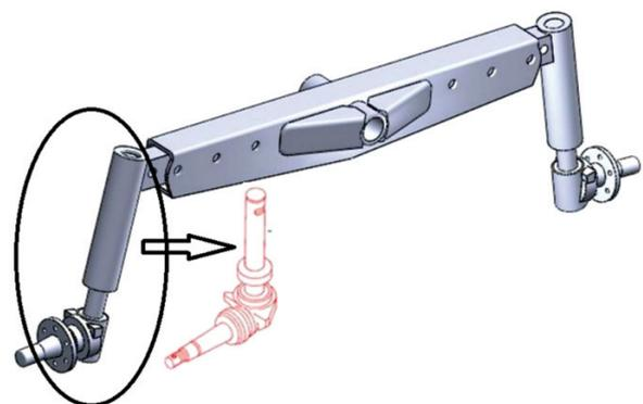
Figure 1: Tractor front axle
