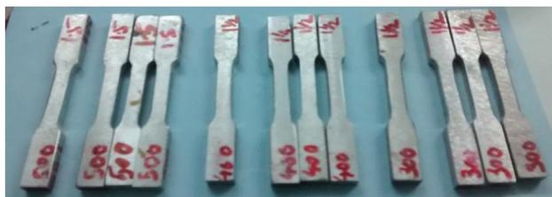
**Figure 3:** Samples before the tensile-strength testing and after annealing at different temperatures (500, 400 and 300) °C and then subjected to different TE steps
