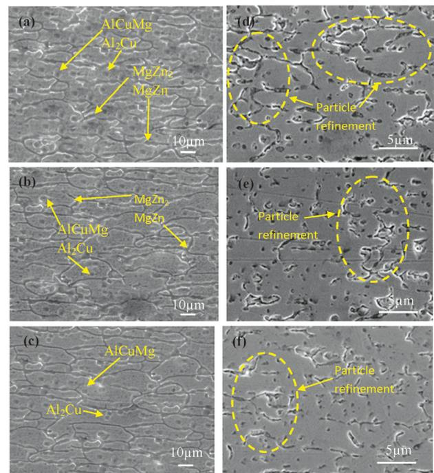
**Figure 7:** SEM surface morphologies of the AA 7075 aluminum alloy in the starting condition prior to TE and after three TE passes: annealed at: a) 300 °C, b) 400 °C, c) 500 °C; and after TE: d) three passes after annealing at 300 °C, e) three passes after annealing at 400 °C, f) three passes after annealing at 500 °C
