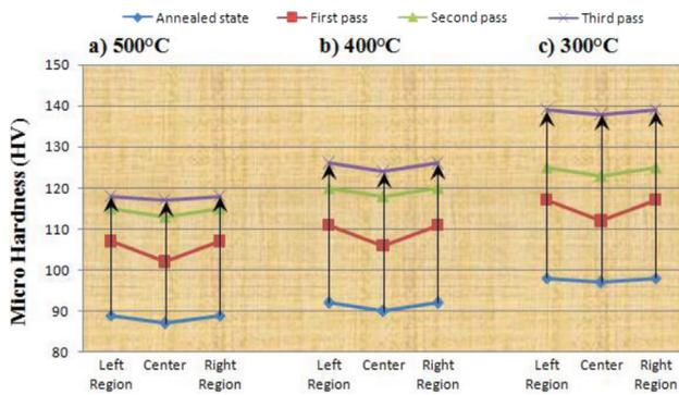
**Figure 5:** Micro-hardness at different locations before and after TE for the billets of the AA 7075 aluminum alloy annealed at different temperatures: a) 500 °C, b) 400 °C and c) 300 °C
