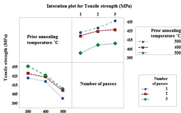
**Figure 4:** Tensile-strength values corresponding to different treatments
