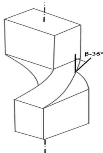
**Figure 2:** Schematic representation of the TE process
