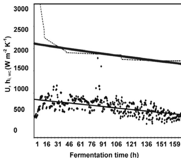
Fig 1: Heat transfer coefficients on 7.5 m<sup>3</sup> scale with A315 impellers
