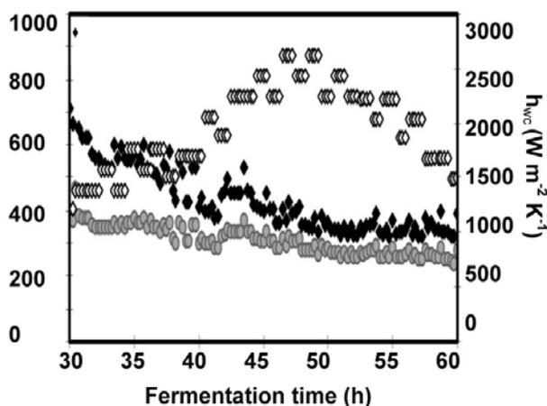
Fig 2: Heat transfer coefficients on 15 m<sup>3</sup> scale with Rushton impellers
