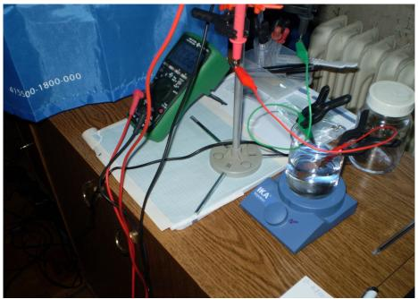
5.4.7.8.2.9.2 Figure 386: Measurement of voltage and current for NaCl solution
