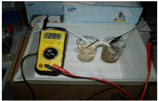
5.5.4.1.3.7 Figure 444: Voltage and current measurements of the soil galvanic cell
