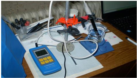
5.4.7.8.2.9 Figure 385: Measurement of NaCl solution conductivity
