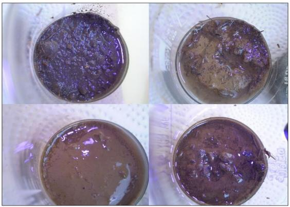
5.5.4.1.3.3 Figure 440: Evaluation of soil density using UV light
