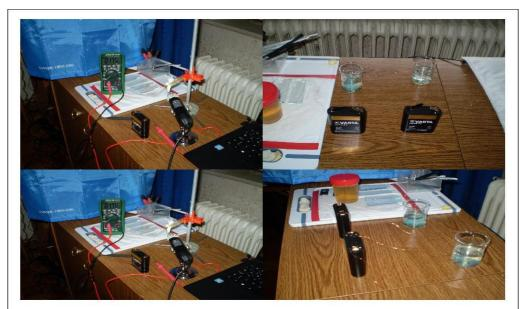
5.4.7.4.2 Figure 348: Electrolysis tests of sugar solution with and without brown algae
