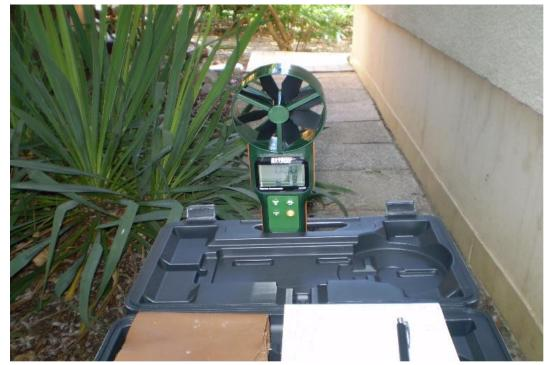
5.6.4.1 Figure 485: Measuring wind speed using an anemometer
