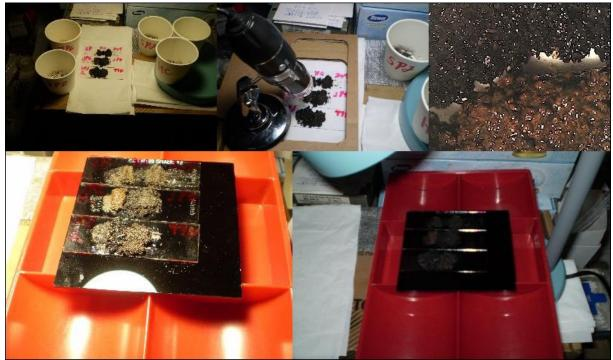
5.5.4.1.4.2.1 Figure 448: Technique for evaluating optical blackness between HC soil and other soils
