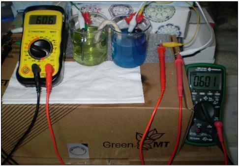
5.4.7.8.9.6 Figure 434: Galvanic cell with saturated solutions of FeSO<sub>4</sub>·7H<sub>2</sub>O and CuSO<sub>4</sub>·5H<sub>2</sub>O
