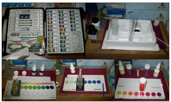
5.5.4.1.4.6.2 Figure 452: Analysis of color and turbidity of soil filtrates
