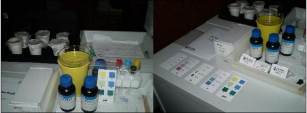
5.5.4.1.4.6 Figure 451: Analysis of colors and turbidity of NPK in soils
