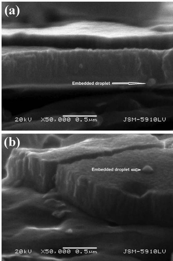
**Figure 4:** SEM (SEI) of micrographs of fractured surface (in liquid nitrogen) of TiN coating from different areas a) and b). Columnar grains of TiN through fractured coating seen at a) and b). Embedded droplets at surface b) and at coating/substrate interface a) were marked.
