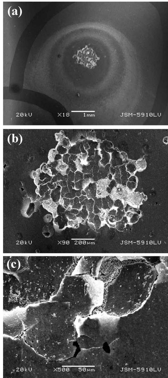
**Figure 10:** SEM (SEI) micrographs taken from the one of the large pits formed during early exposure: a) the micrograph of the pit marked at low magnification, b) the micrograph from the interior of the pit and c) the micrograph from the periphery of the pit interior at high magnification
