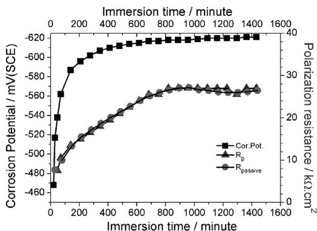
**Figure 13:** The corrosion potential (Cor.Pot.), polarization resistance ( $R_p$  and  $R_{\text{passive}}$  calculated from EIS data) for the substrate in 3 % NaCl solution as a function of immersion time
