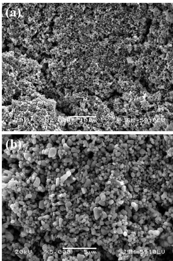
**Figure 11:** SEM (SEI) micrographs taken from the interior of the pit in **Figure 10** where the scale was removed: a) low magnification and b) high magnification from the same area in a). Equiaxed particles were observed on substrate surface at a) and b).
