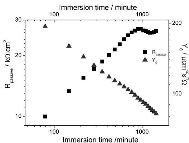
**Figure 14:** The admittance ( $Y_0$ ) and polarization resistance ( $R_{passive}$  calculated from EIS data) for the substrate in 3 % NaCl solution as a function of immersion time
