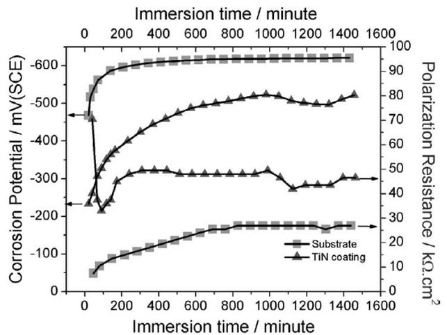
**Figure 5:** Corrosion potentials and polarization resistances ( $R_p$ ) of the substrate and TiN-coated substrates determined from the polarization resistance scan (Figures 6 and 7) in 3 % NaCl solution as a function of the immersion time
