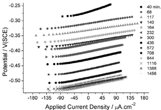
**Figure 7:** Polarization resistance scan of TiN coating in 3 % NaCl solution as a function of immersion time
