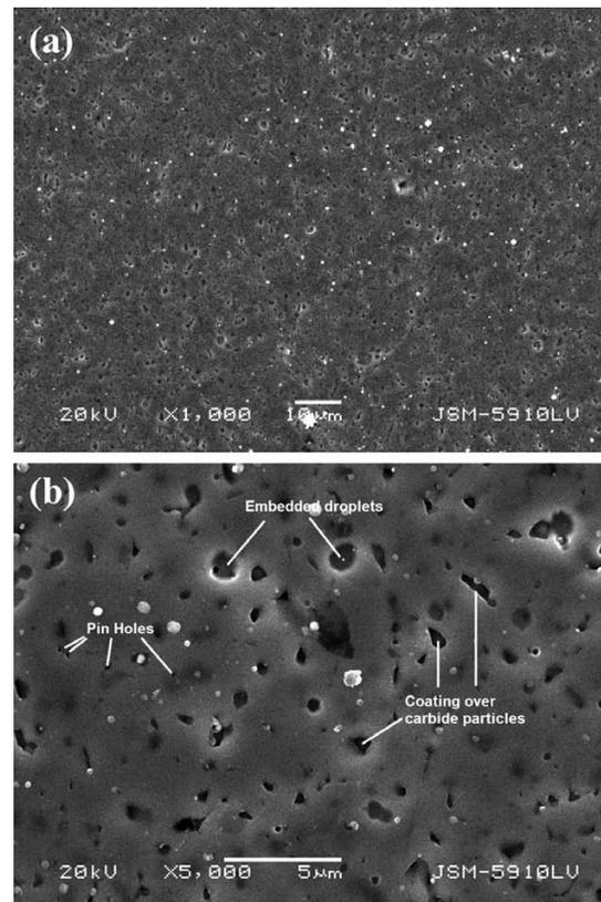
**Figure 3:** SEM (SEI) micrographs taken from TiN-coating surface at: a) low magnification and b) high magnification. TiN coating deposited over carbide phases (dark areas) were distinguished with depression over the surface at a) and b). Embedded droplets deposited throughout the surface were marked at b). Bright particles on coating surface were un-embedded droplets (spherical particles). Pin holes were marked on surface b).
