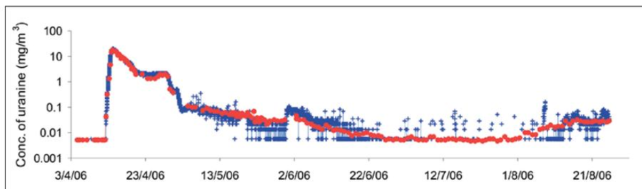
Fig. 4: Parallel measurements with field-fluorometer LLF-M (blue) and Luminescence Spectrometer LS 30 (red) coincide well.
