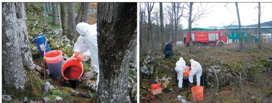
Fig. 6: Injections of eosin (left) and uranine (right) on April 5, 2006 (Photo: M. Petrič).
