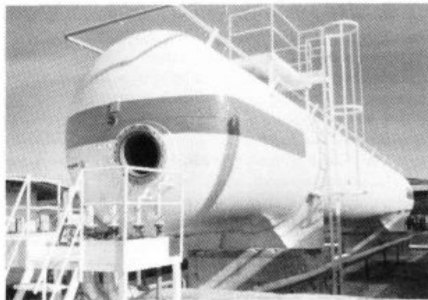
Slika 1: Horizontalna stabilna tlačna posoda prostornine 150 m 3 Figure 1: Horizontal stable pressure vessel of volume 150 m 3
