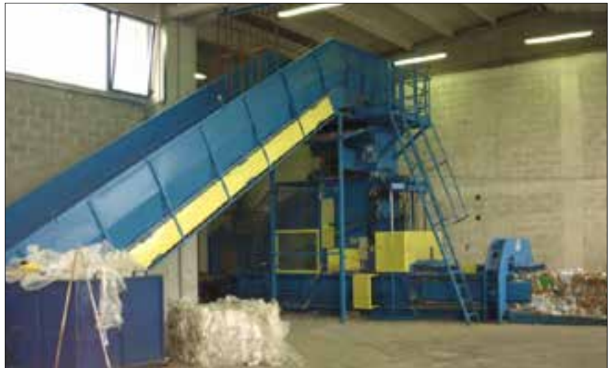
Figure 3. Horizontal bailer press with feeding system
